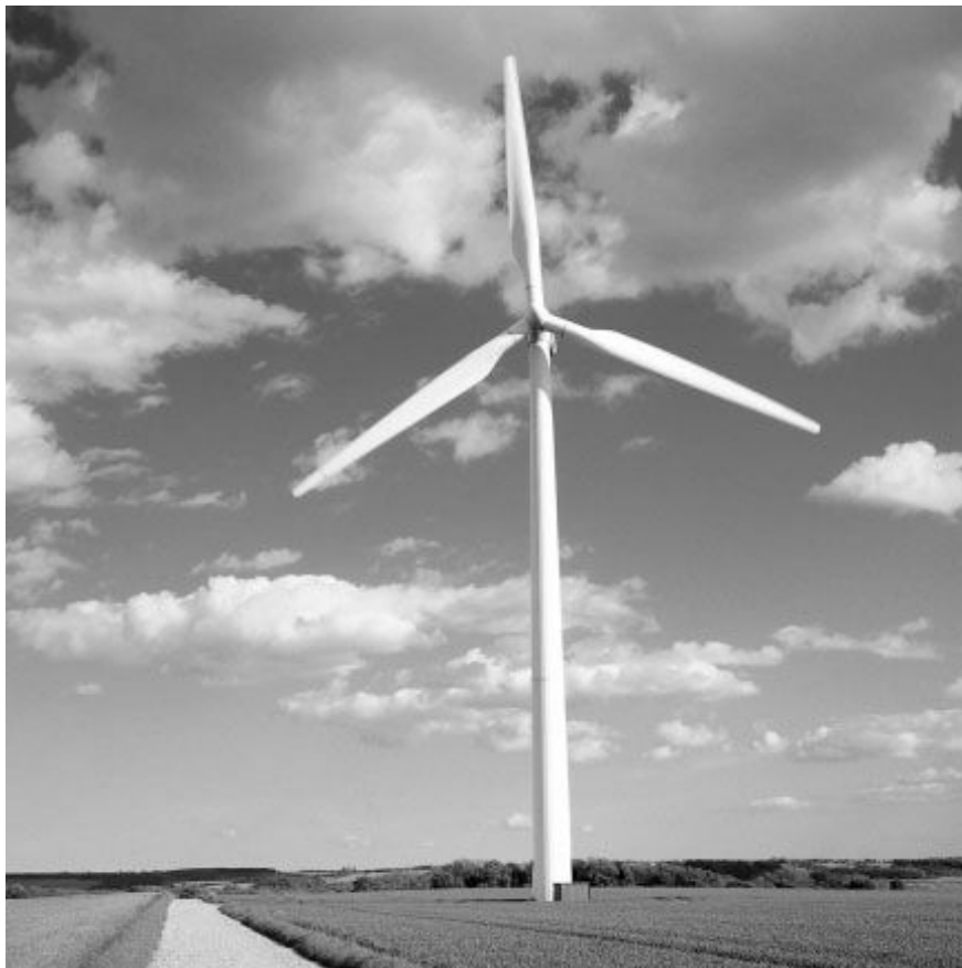
Figure 1.2: 750 kW, 48 m diameter Wind Turbine, Denmark (Reproduced by permission of NEG MICON)
