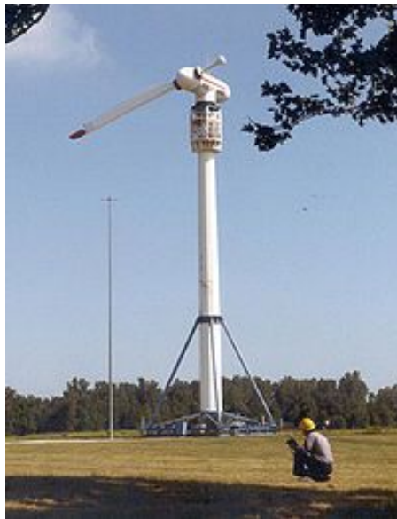
Figure 3.3: The NASA Mod-0 research wind turbine at Glenn Research Center's Plum Brook station in Ohio tested a one-bladed rotor configuration
