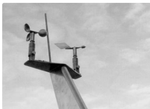
Figure2.9: Cup anemometer for wind speed indication (left) * Lightning conductor (middle) * Wind direction indicator (right)
