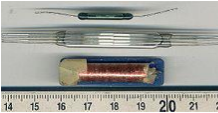
Fig: Top, middle: reed switches, bottom: reed relay
