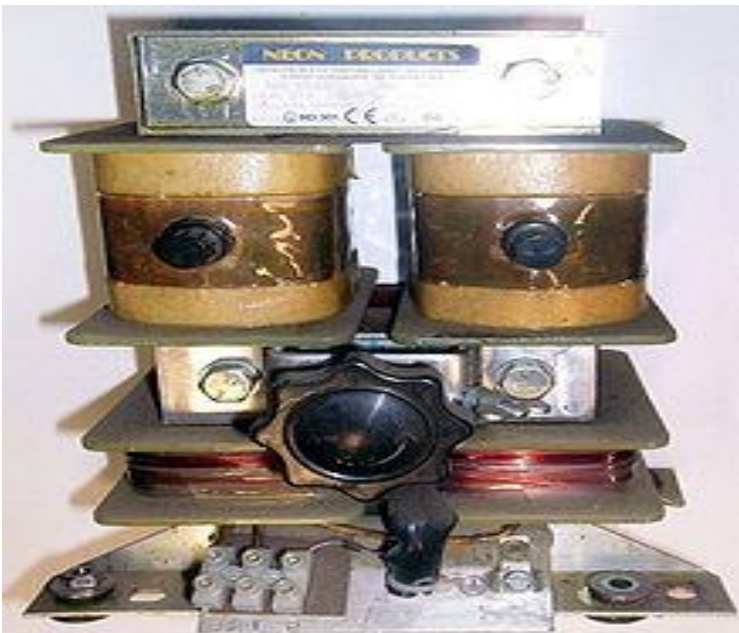
Fig: Leakage transformer
