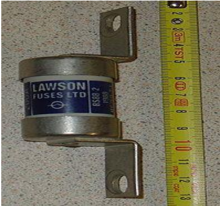
Fig: 200 A Industrial fuse. 80 kA breaking capacity.
