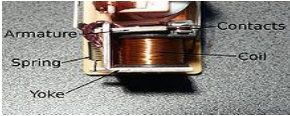
Fig: Simple electromechanical relay
