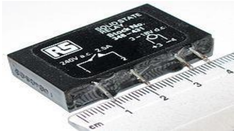
Fig: Solid state relay, which has no moving parts
