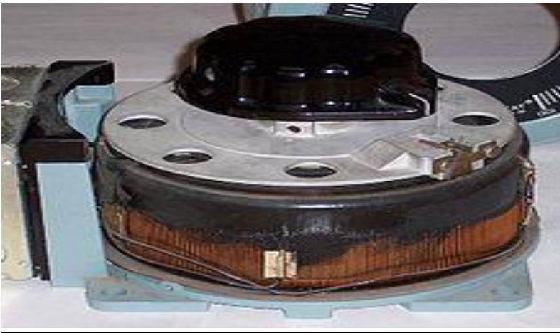
Fig: An autotransformer with a sliding brush contact
