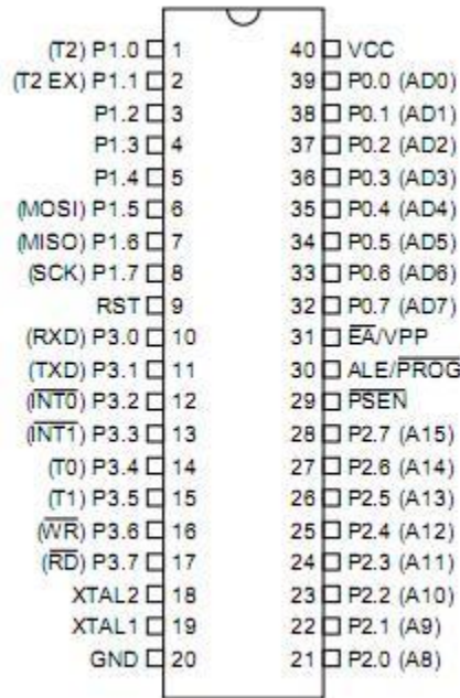
Figure - 4.2 : Pin configuration of AT89S52
