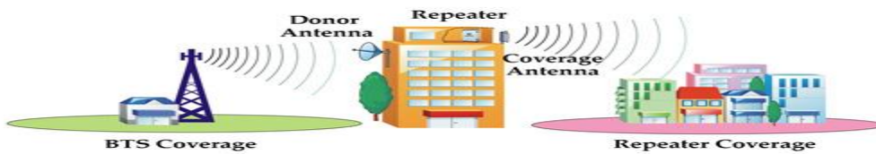
Fig:4.9.a Application Diagram of Outdoor Single-Band RF Repeater
