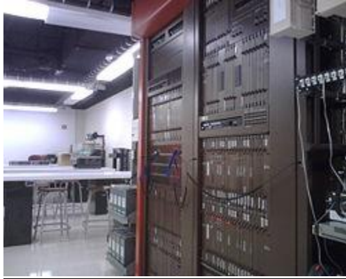
Figure: A DMS-10 used as a lab trainer at Southeast Missouri State University.
