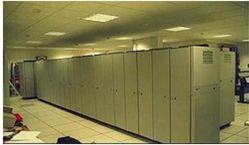
Figure: A DMS-250 used by an operator to offer local and long distance services in France.
