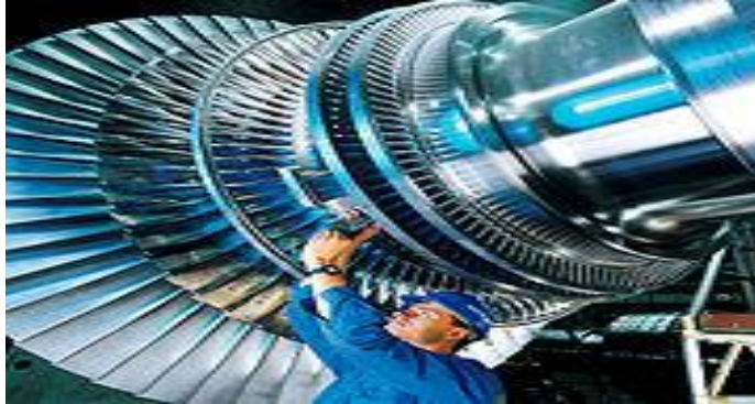
Fig 4-2: A rotor of a modern steam turbine, used in a power plant
