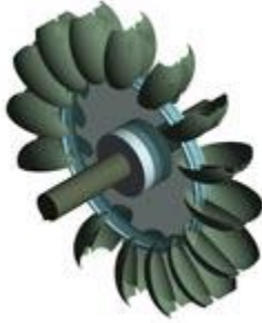
Fig 4-4: runner and bucket of impulse turbine.
