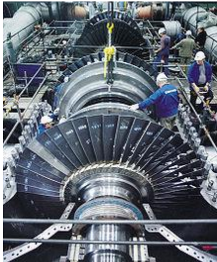
Fig4-1: A Siemens steam turbine with the case opened.
