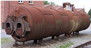
Fig 5-3: An industrial boiler, originally used for supplying steam to a stationary steam engine
