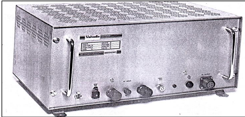
Figure 3.18: Example of a solid-state power inverter. From a 24V d.c. input, this inverter provides 240 V sinusoidal a.c. output with a rating of 100 W. The weight of the unit is 37.3 kg (17 lb). (Source Valradio Power Ltd.)
