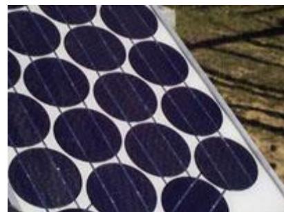
Fig-2.5: Single-Crystal Cells
