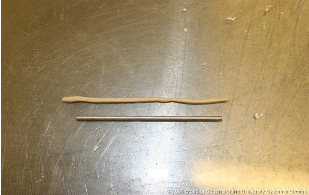
Picture 9: Plastic limit determination
