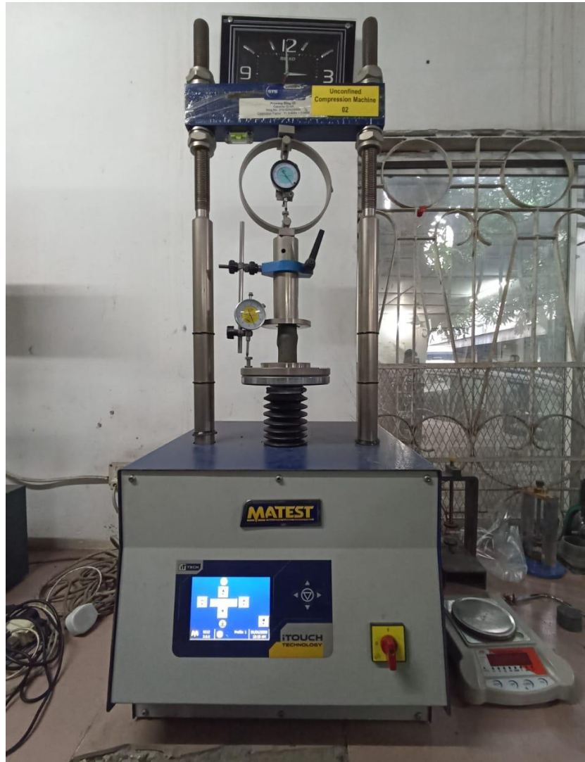
Picture 10: Unconfined Compressive Strength Test
