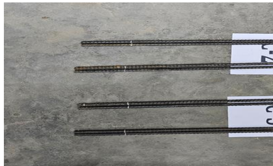
Figure 3.15: Grip length mark of sample
