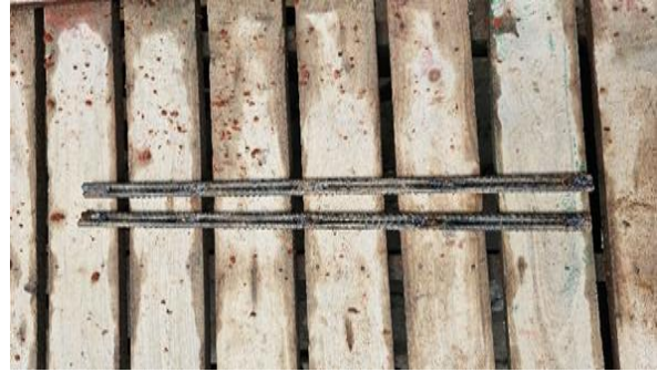
Figure 3.12: C-1 Welded sample
