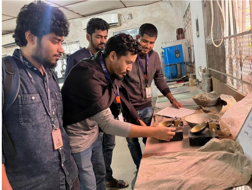
Picture 7: Liquid Limit Test
