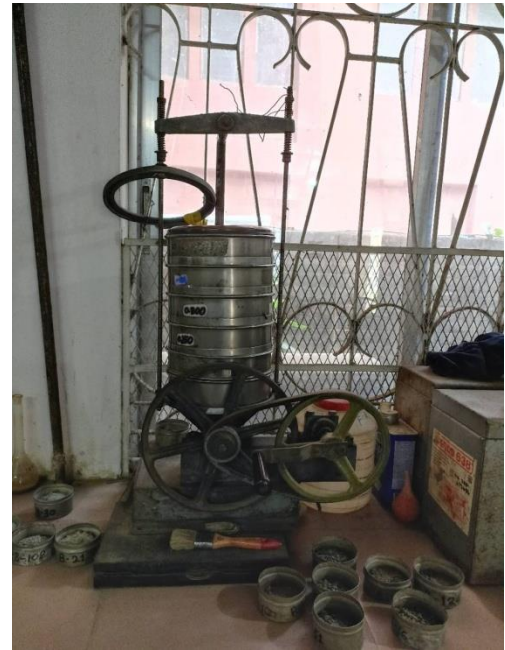
Picture 4: Grain Size Analysis by Sieve Analysis
