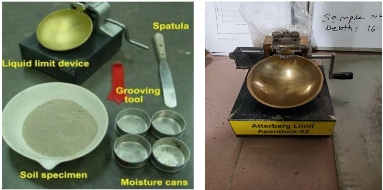
Picture 8: Apparatus of liquid limit determination
