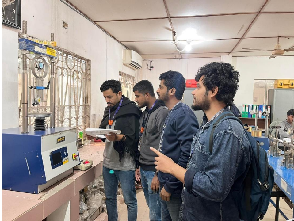
Picture 11: Unconfined Compressive Strength Test
