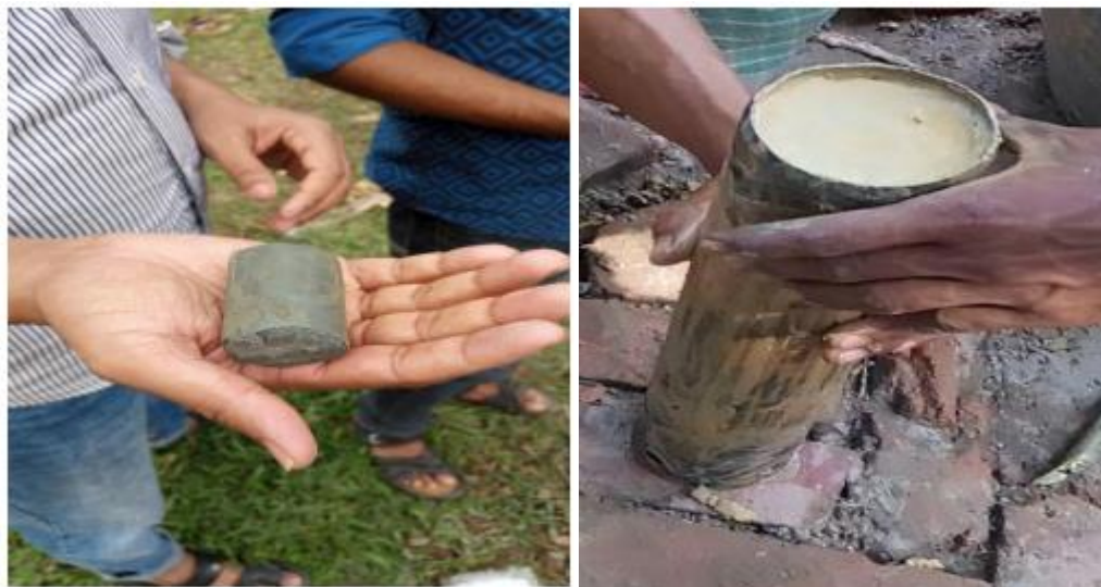
Picture 3: Soil sample collection from split spoon sampler
