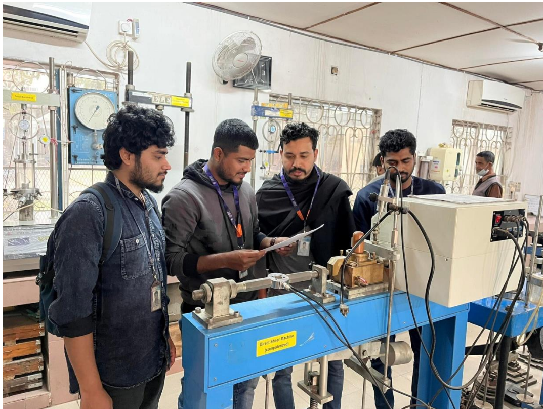
Picture 13: Direct Shear Test
