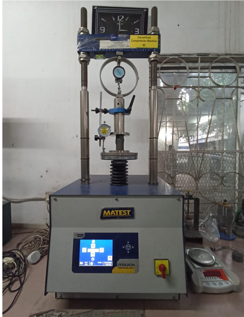
Picture 10: Unconfined Compressive Strength Test
