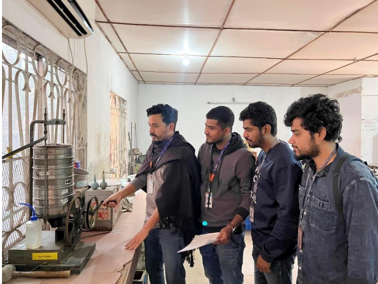
Picture 4: Grain Size Analysis by Sieve Analysis
