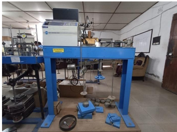
Picture13: Direct Shear
