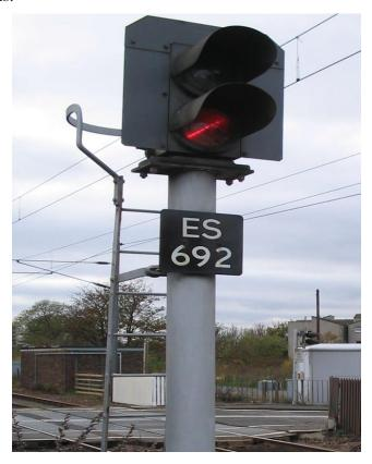
Photo: 5.2 Network Rail (UK) two-aspect color light railway signal set at 'danger'
