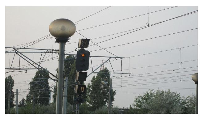
**Photo: 5.3** Railway signal in Ploiesti West railway station, Romania. This type of signal is based on the German Ks signals.
