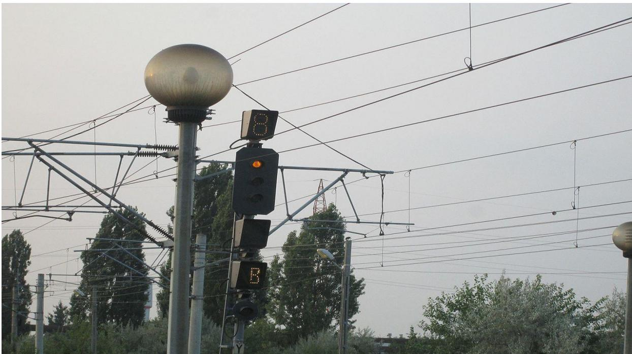
**Photo: 5.3** Railway signal in Ploiesti West railway station, Romania. This type of signal is based on the German Ks signals.
