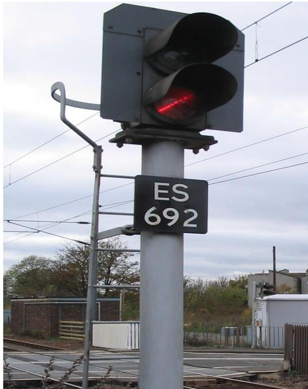
**Photo: 5.2** Network Rail (UK) two-aspect color light railway signal set at 'danger'
