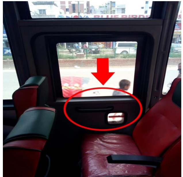
Photo 4.44: Emergency Exit Door
