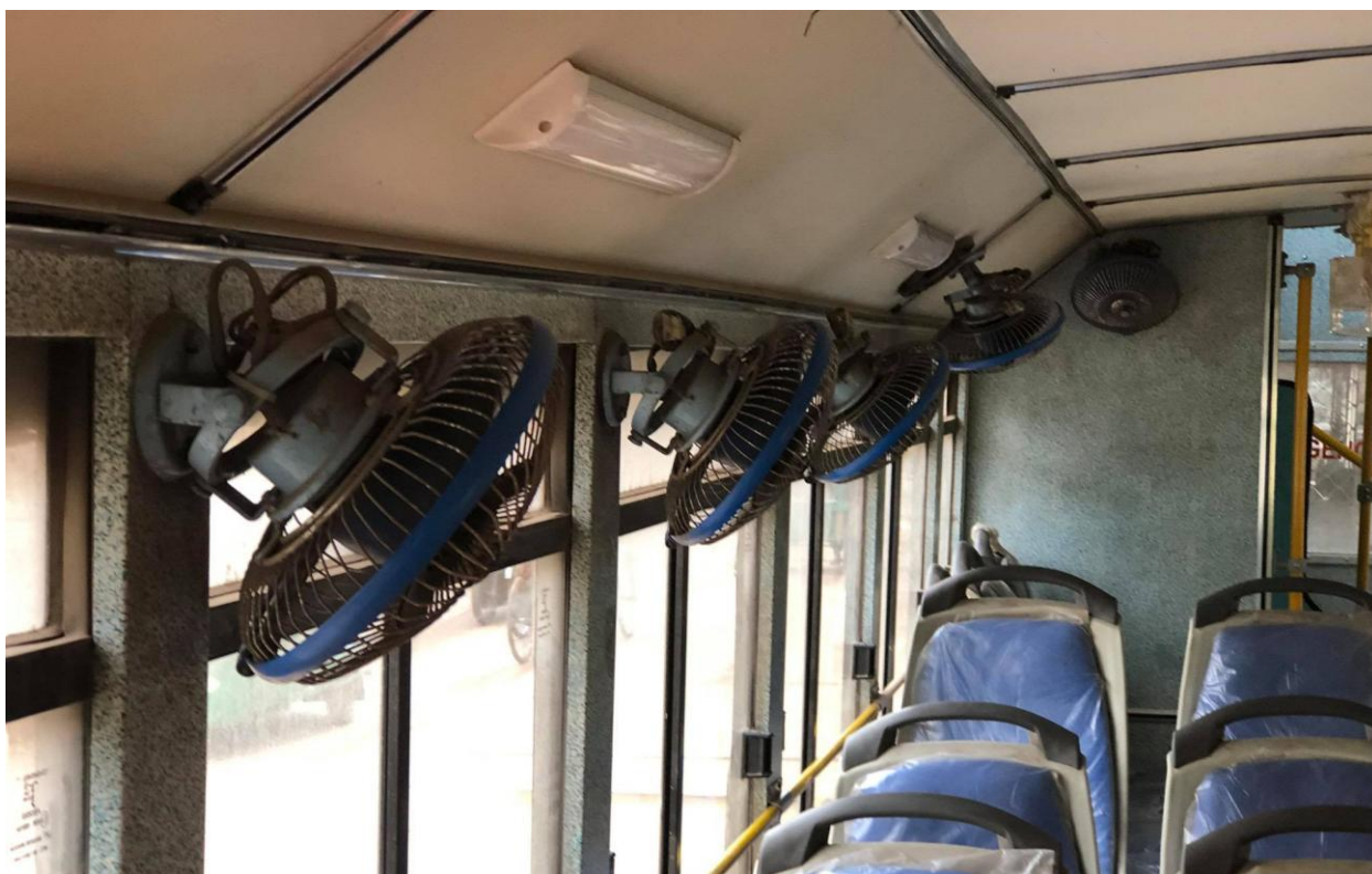
Photo 4.11: BRTC Bus (Fan & Light Facilities)
