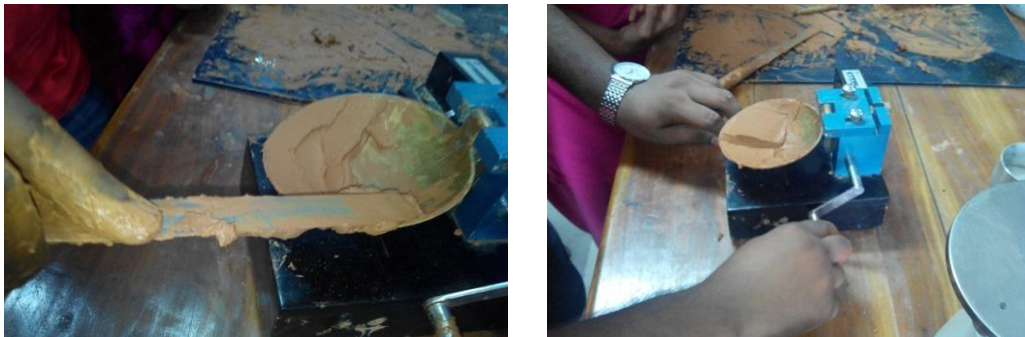
Figure 3.3: Atterberg Limit Test.
