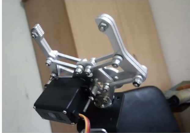
Figure 3.2: Gripper Connecting with servo motor
