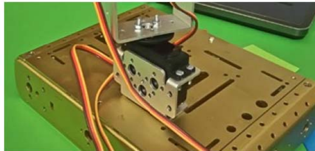
Figure 3.4: Robot base Connecting with servo motor
