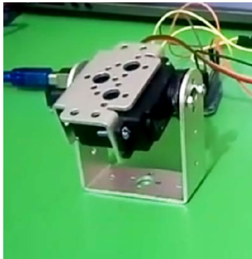
Figure 3.3: Wrist Connecting with servo motor
