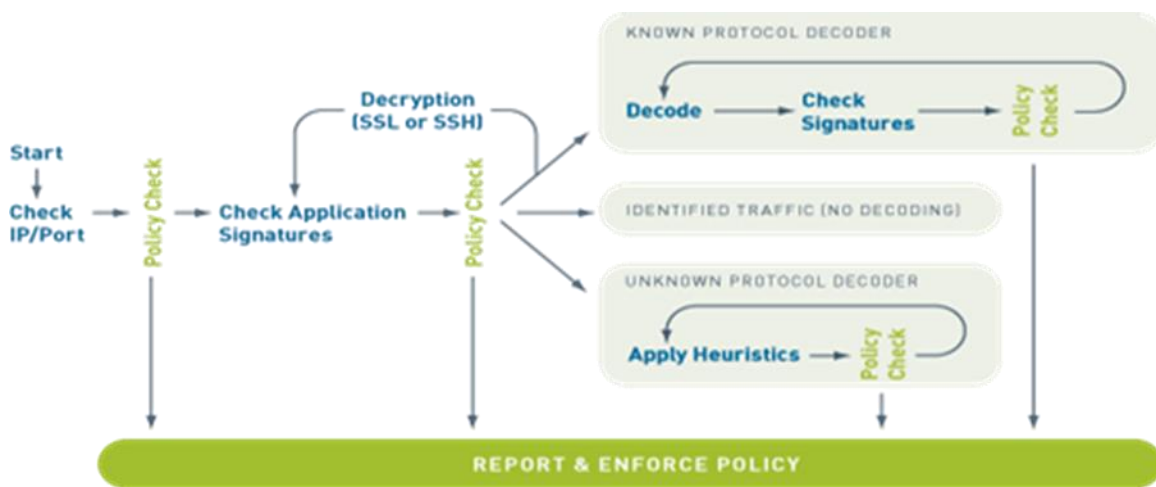
Figure 4.8: Functional Procedure of DMZ Firewall
