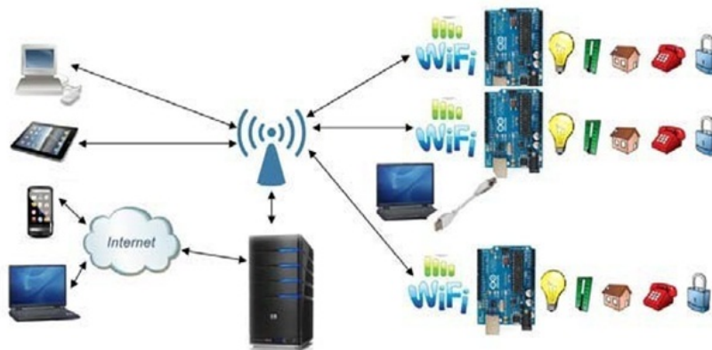
Figure 2.5: The proposed home automation system layout
