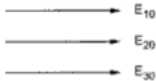
Fig. 1.5(a) Zero phase sequence
