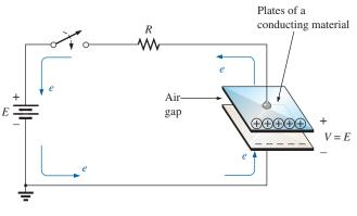
FIG. 10.4 Fundamental charging circuit.
