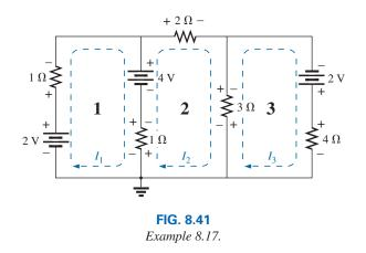
**Solution:** Each window is assigned a loop current in the clockwise direction:
