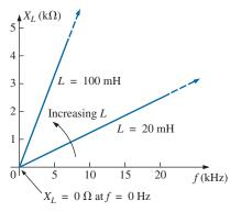
**FIG. 14.20** *X<sub>L</sub> versus frequency.*
