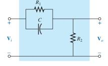
**FIG. 21.68** *High-pass filter with limited attenuation.*
