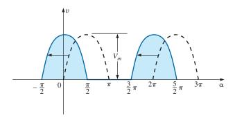
**FIG. 25.18** *Changing the phase angle of a waveform.*
