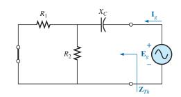
FIG. 18.45 Determining the Thévenin impedance for the network in Fig. 18.41 using the approach  $Z_{Th} = E_g/I_g$ .
