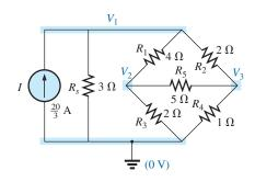
FIG. 8.72 Defining the nodal voltages for the network in Fig. 8.70.
