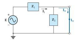
**FIG. 18.65** Determining  $I_N$  for the network in Fig. 18.62.
