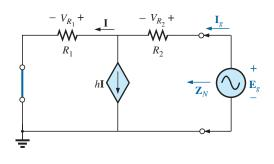
FIG. 18.80 Determining the Norton impedance using the approach  $\mathbf{Z}_N = \mathbf{E}_g / \mathbf{E}_g$ .
