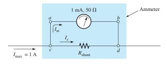
FIG. 7.49 Basic ammeter.
