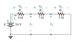
**FIG. 5.82** Series dc network to be analyzed using PSpice.
