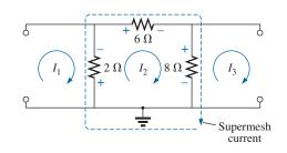
FIG. 8.38 Defining the supermesh current for the network in Fig. 8.36.
