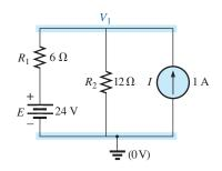
**FIG. 8.47** *Network in Fig. 8.46 with assigned nodes.*
