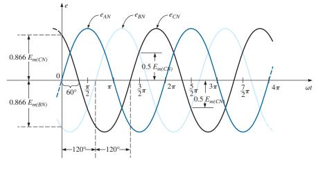
**FIG. 23.2** *Phase voltages of a three-phase generator.*
