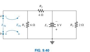
Determining  $E_{Th}$  for the network in Fig. 9.38.
