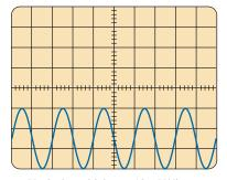
Vertical sensitivity = 10 mV/div. Horizontal sensitivity = 0.2 ms/div.
