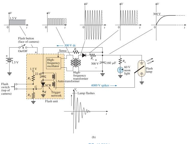
FIG. 10.78(b) Flash camera: basic circuitry.
