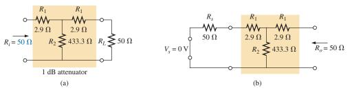
**FIG. 21.87** *1 dB attenuator: (a) loaded; (b) finding*  $R_a$ .
