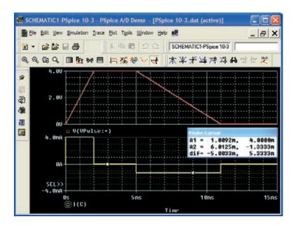
**FIG. 10.86** *The applied pulse and resulting current for the 2*  $\mu$ *F capacitor in Fig. 10.85.*
