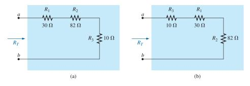
FIG. 5.8 Two series combinations of the same elements with the same total resistance.
