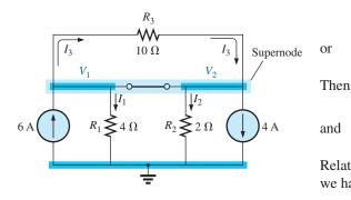
**FIG. 8.58** Defining the supernode for the network in Fig. 8.57.
