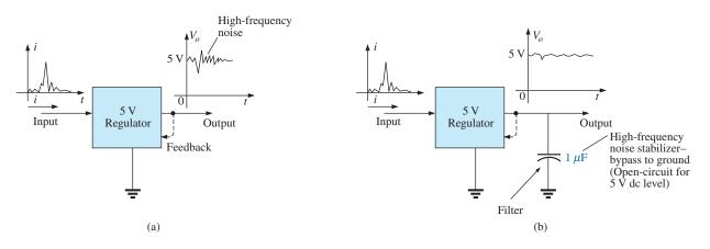
**FIG. 21.92** *Regulator:* (a) effect of spike in current on the input side; (b) noise reduction.
