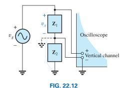
Demonstrating the shorting effect introduced by the grounded side of the vertical channel of an oscilloscope.
