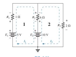
**FIG. 8.39** Network in Fig. 8.31 redrawn with assigned loop currents.
