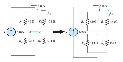
**FIG. 9.16** *The effect of the current source I on the current I*<sub>2</sub>*.*
