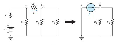
FIG. 9.105 Demonstrating the effect of knowing a current at some point in a complex network.
