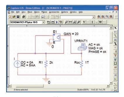
FIG. 18.101 Using PSpice to determine the open-circuit Thévenin voltage for the network in Fig. 18.51.
