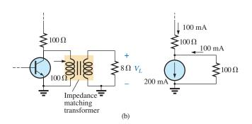
FIG. 18.94 (a) Network in Fig. 18.93 following the substitution of the transistor equivalent network; (b) effect of the matching transformer.
