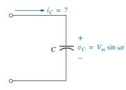
FIG. 14.11 Investigating the sinusoidal response of a capacitive element.
