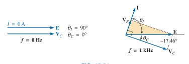
**FIG. 15.51** The phasor diagram for the circuit in Fig. 15.47 for f = 0 Hz and 1 kHz.
