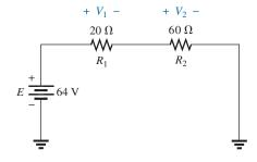
**FIG. 5.37** Series circuit to be examined using the voltage divider rule in Example 5.15.
