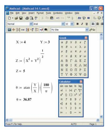
FIG. 14.68 Using Mathcad to convert from rectangular to polar form.
