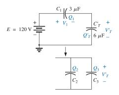
**FIG. 10.72** *Reduced equivalent for the network in Fig. 10.71.*
