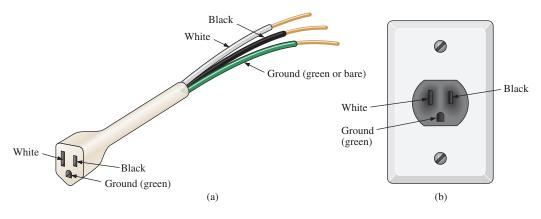
FIG. 16.25 Three-wire conductors: (a) extension cord; (b) home outlet.
