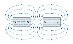
**FIG. 11.3** *Flux distribution for two adjacent, like poles.*
