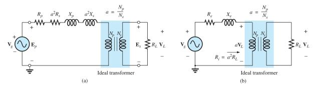
FIG. 22.18 Reflecting the secondary circuit into the primary side of the iron-core transformer.
