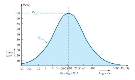
**FIG. 9.81**  $P_L$  versus  $R_L$  for the network in Fig. 9.79.
