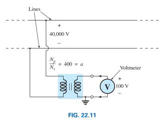
Isolating a high-voltage line from the point of measurement.
