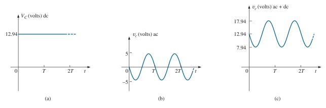
**FIG. 18.95** Collector voltage for the network in Fig. 18.91: (a) dc; (b) ac; (c) dc and ac.
