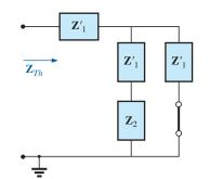
FIG. 18.88 Determining  $\mathbf{Z}_{Th}$  for the network in Fig. 18.85.
