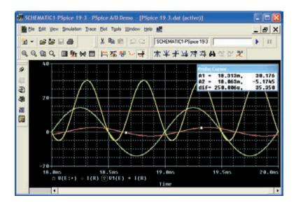
**FIG. 19.43** Plots of the applied voltage e, current  $i_R = i_s$ , and power delivered  $p_s = e \cdot i_s$ for the circuit in Fig. 19.42.
