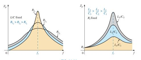
**FIG. 20.28** *Effect of*  $R_1$ , L, and C on the parallel resonance curve.
