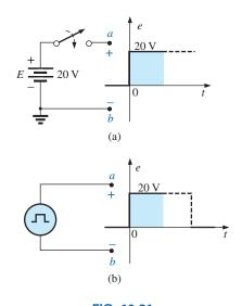
FIG. 10.81 Establishing a switching dc voltage level: (a) series dc voltage-switch combination; (b) PSpice pulse option.
