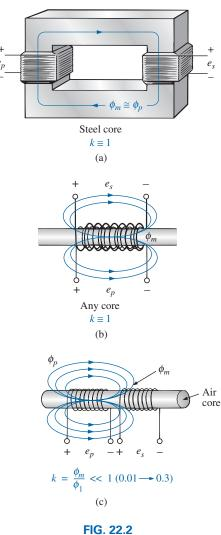
Windings having different coefficients of coupling.
