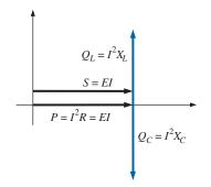
FIG. 20.4 Power triangle for the series resonant circuit at resonance.
