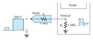
**FIG. 24.36** ×10 attenuator probe.
