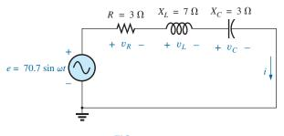
FIG. 15.35 Series R-L-C ac circuit.
