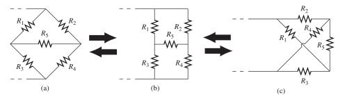
**FIG. 8.69** Various formats for a bridge network.
