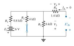
**FIG. 9.51** Determining the contribution to  $E_{Th}$  from the source  $E_1$  for the network in Fig. 9.49.
