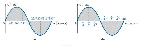
FIG. 13.15 Plotting a sine wave versus (a) degrees and (b) radians.
