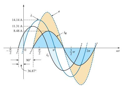
FIG. 15.76 Waveforms for the parallel R-C network in Fig. 15.72.
