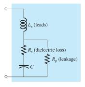
**FIG. 14.27** *Practical equivalent for a capacitor.*
