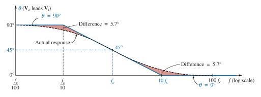
FIG. 21.47 Phase response for a high-pass R-C filter.
