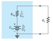
**FIG. 9.94** *Converting the current source in Fig. 9.93 to a voltage source.*
