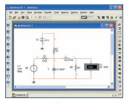
**FIG. 18.105** Using Multisim to apply superposition to the network in Fig. 18.12.
