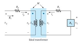
FIG. 22.31 Air-core transformer equivalent circuit.
