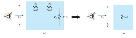
FIG. 5.13 Resistance "seen" at the terminals of a series circuit.
