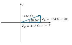
**FIG. 15.64** Impedance diagram for the network in Fig. 15.63.
