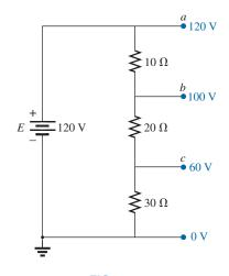
**FIG. 7.39** *Voltage divider supply.*
