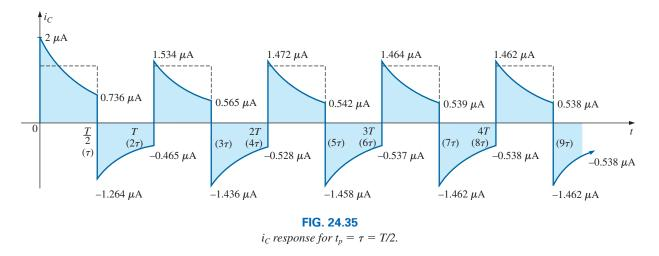
For the trailing edge of the first pulse, the voltage across the capacitor cannot change instantaneously, resulting in the following when  $v_i$  drops to zero volts:
