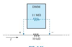
FIG. 6.61 Voltmeter loading.
