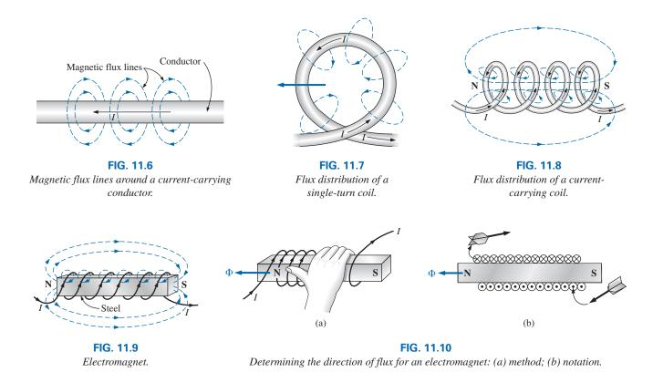
single-turn coil (Fig. 11.7), the resulting flux flows in a common direction through the center of the coil. A coil of more than one turn produces a magnetic field that exists in a continuous path through and around the coil (Fig. 11.8).
