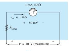
FIG. 7.51 Basic voltmeter.
