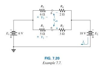
**Solutions:** This is one of those situations where it may be best to redraw the network before beginning the analysis. Since combining both sources will not affect the unknowns, the network is redrawn as shown in Fig. 7.21, establishing a parallel network with the total source voltage across each parallel branch. The net source voltage is the difference between the two with the polarity of the larger.
