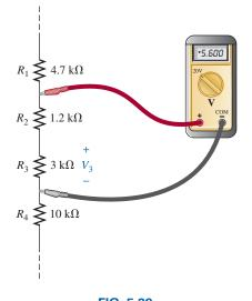
**FIG. 5.39** *Voltage divider action for Example 5.18.*
