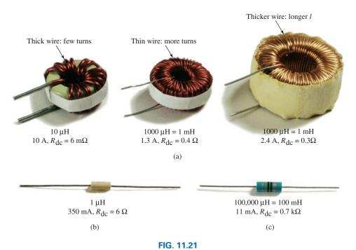
Relative sizes of different types of inductors: (a) toroid, high-current; (b) phenolic (resin or plastic core); (c) ferrite core.
