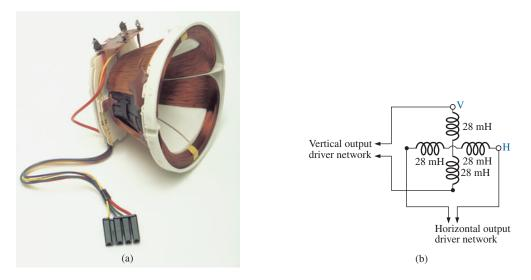
**FIG. 11.71** (a) Black-and-white TV yolk assembly; (b) schematic representation.
