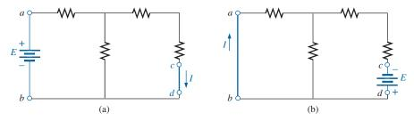
**FIG. 9.106** Demonstrating the impact of the reciprocity theorem.
