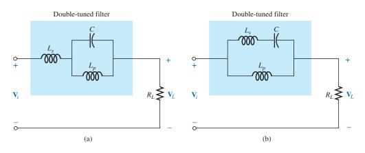
**FIG. 21.43** *Double-tuned networks.*
