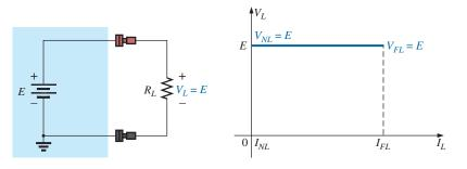
**FIG. 5.69** *Ideal supply and its terminal characteristics.*
