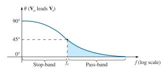
**FIG. 21.24** *Phase-angle response for the high-pass R-C filter.*
