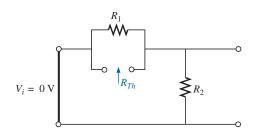
**FIG. 21.69** Determining R for the  $f_c$  calculation for the filter in Fig. 21.68.
