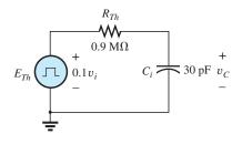
**FIG. 24.39** *Thévenin equivalent for*  $C_i$  *in Fig. 24.38.*
