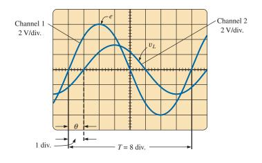
**FIG. 15.107** Determining the phase angle between e and  $v_L$  for the configuration in Fig. 15.106.
