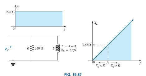
The frequency response of the individual elements of a parallel R-L network.
