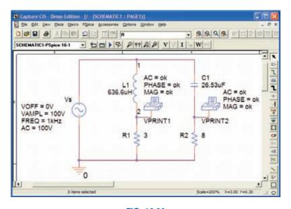
**FIG. 16.30** Determining the voltage across  $R_1$  and  $R_2$  using the **VPRINT** option of a *PSpice analysis.*
