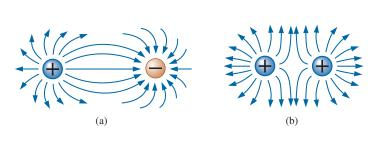
FIG. 10.3 Electric flux distributions: (a) opposite charges; (b) like charges.
