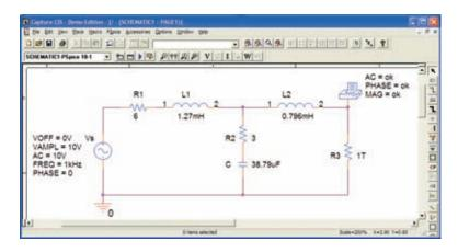
FIG. 18.97 Using PSpice to determine the open-circuit Thévenin voltage.
