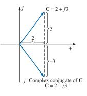
FIG. 14.53 Defining the complex conjugate of a complex number in rectangular form.
