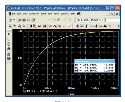
FIG. 10.84 Transient response for the voltage across the capacitor in Fig. 10.80 when VPulse is applied.
