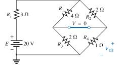
FIG. 8.76 Substituting the short-circuit equivalent for the balance arm of a balanced bridge.
