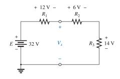
FIG. 5.28 Series dc circuit to be analyzed in Example 5.9.
