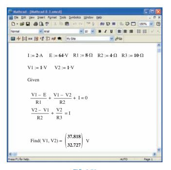
FIG. 8.53 Using Mathcad to verify the mathematical calculations of Example 8.20.
