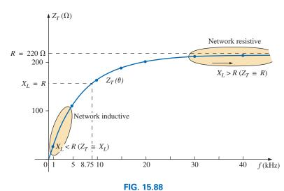
The magnitude of the input impedance versus frequency for the network in Fig. 15.86.
