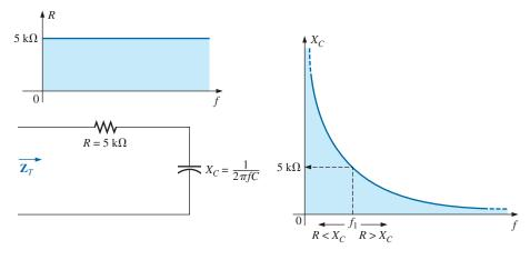
**FIG. 15.48** The frequency response for the individual elements of a series R-C circuit.
