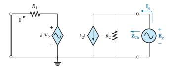
**FIG. 18.59** Determining  $\mathbf{Z}_{Th}$  using the procedure  $\mathbf{Z}_{Th} = \mathbf{E}_g / \mathbf{I}_g$ .
