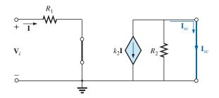
**FIG. 18.58** Determining  $I_{sc}$  for the network in Fig. 18.57.
