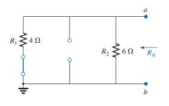
**FIG. 9.74** Determining  $R_N$  for the network in Fig. 9.73.
