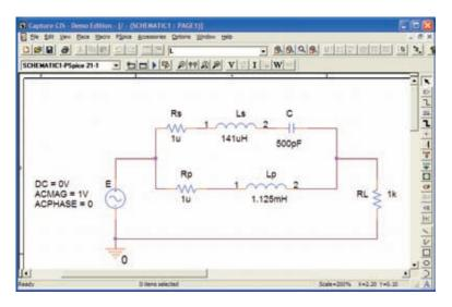
FIG. 21.93 Using PSpice to analyze a double-tuned filter.
