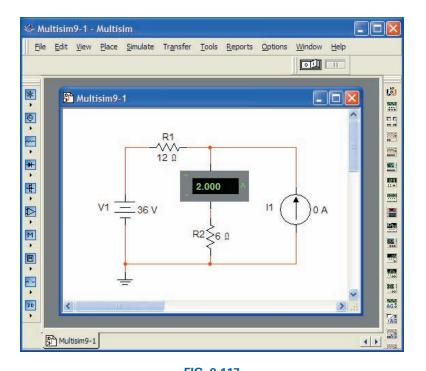
FIG. 9.117 Using Multisim to determine the contribution of the 36 V voltage source to the current through  $R_2$ .
