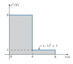
FIG. 13.61 The squared waveform of Fig. 13.60.
