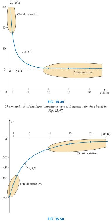
The phase angle of the input impedance versus frequency for the circuit in Fig. 15.47.
