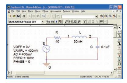
FIG. 20.42 Series resonant circuit to be analyzed using PSpice.
