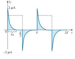
**FIG. 24.33** *i<sub>c</sub> for the R-C network in Fig. 24.31.*
