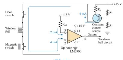
FIG. 8.96 Constant current alarm system with electronic components.
