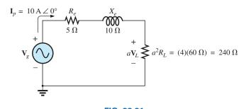
FIG. 22.21 Transformed equivalent circuit of Fig. 22.20.
