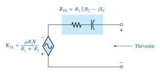
**FIG. 18.46** *The Thévenin equivalent circuit for the network in Fig. 18.41.*
