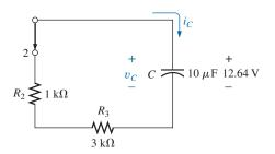
**FIG. 10.48** Network in Fig. 10.47 when the switch is moved to position 2 at  $t = 1\tau_1$ .
