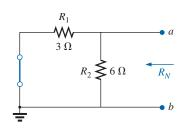
**FIG. 9.63** *Determining*  $R_N$  *for the network in Fig. 9.62.*
