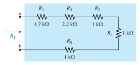
FIG. 5.10 Series circuit of Fig. 5.9 redrawn to permit the use of Eq. (5.2):  $R_T = NR$ .
