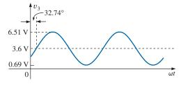
FIG. 18.17 The resultant voltage  $v_3$  for the network in Fig. 18.12.
