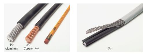
FIG. 4.25 200 A service conductors: (a) 4/0 aluminum and 2/0 copper; (b) three-wire 4/0 aluminum service.
