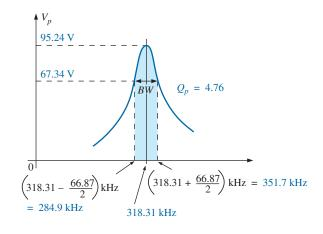
FIG. 20.37 Resonance curve for the network in Fig. 20.36.
