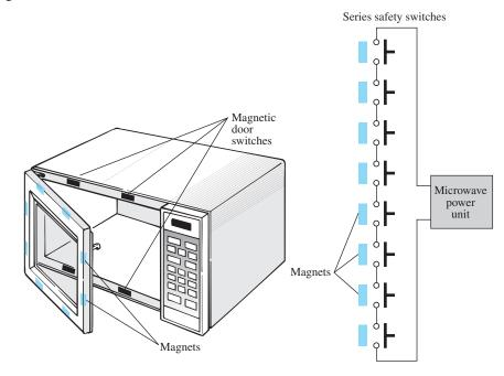
FIG. 5.80 Series safety switches in a microwave oven.
