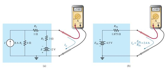
FIG. 9.57 Determining  $R_{Th}$  using the short-circuit current: (a) actual network; (b) Thévenin equivalent.
