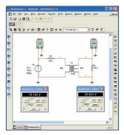
The rest of the configuration is constructed using techniques described earlier. A simulation results in the meter displays in Fig. 22.55. Changing the rms reading of 20.893 V to a peak value results in 29.54 V which is a close match to that obtained using PSpice.
