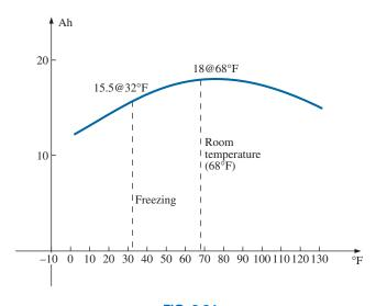
**FIG. 2.24** *Ampere-hour rating (capacity) versus temperature for an Energizer*® *D cell.*
