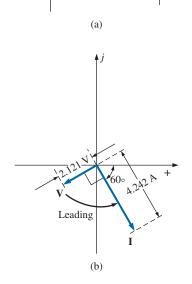
FIG. 15.18 Phasor diagrams for Examples 15.5 and 15.6.
