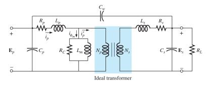
FIG. 22.15 Equivalent circuit for the practical iron-core transformer.
