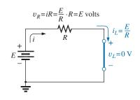
FIG. 11.35 Circuit in Fig. 11.31 under steady-state conditions.
