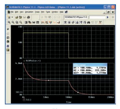
**FIG. 11.79** A plot of the applied pulse and resulting current for the circuit in Fig. 11.78.
