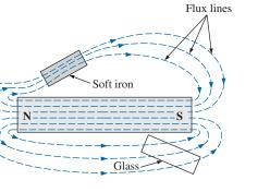
FIG. 11.4 Effect of a ferromagnetic sample on the flux distribution of a permanent magnet.
