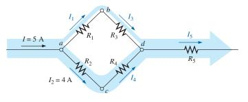
**FIG. 6.34** *Four-node configuration for Example 6.17.*
