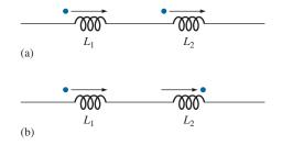
FIG. 22.27 Dot convention for the series coils in (a) Fig. 22.25 and (b) Fig. 22.26.
