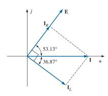
FIG. 15.71 Phasor diagram for the parallel R-L network in Fig. 15.68.
