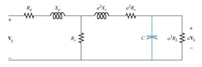
FIG. 22.23 High-frequency reflected equivalent circuit.
