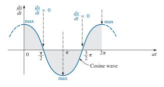
**FIG. 14.2** Derivative of the sine wave of Fig. 14.1.
