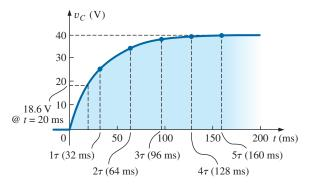
**FIG. 10.37** Plotting the waveform in Fig. 10.36 versus time (t).
