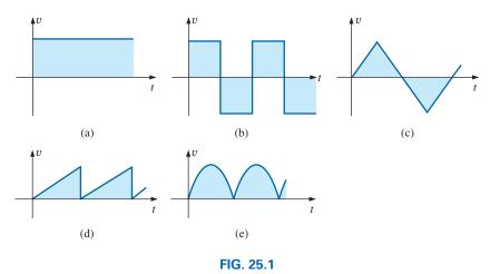
Common nonsinusoidal waveforms: (a) dc; (b) square-wave; (c) triangular; (d) sawtooth; (e) rectified.
