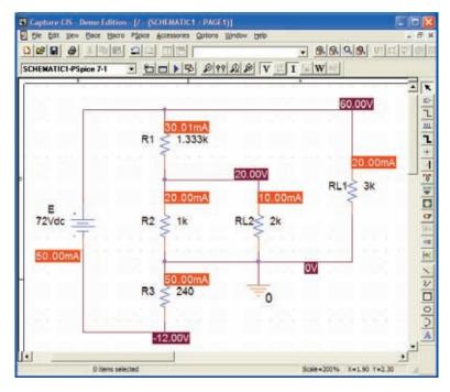
FIG. 7.60 Using PSpice to verify the results of Example 7.12.
