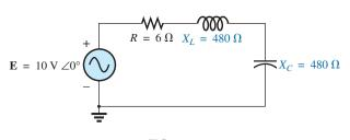
FIG. 20.7 High-Q series resonant circuit.
