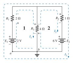
FIG. 8.30 Defining the mesh currents for a "two-window" network.
