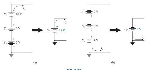
FIG. 5.23 Reducing series dc voltage sources to a single source.
