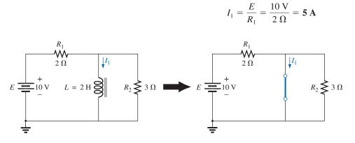
**FIG. 11.60** Substituting the short-circuit equivalent for the inductor for  $t > 5\tau$ .
