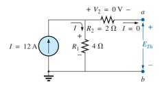
FIG. 9.35 Determining  $E_{Th}$  for the network in Fig. 9.33.
