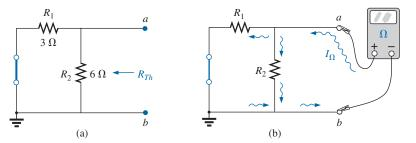
**FIG. 9.28** Determining  $R_{Th}$  for the network in Fig. 9.27.
