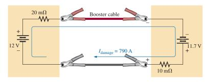
**FIG. 7.58** *Current levels if the booster battery is improperly connected.*
