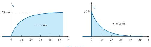
**FIG. 11.37**  $i_L$  and  $v_L$  for the network in Fig. 11.36.
