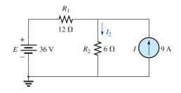
**FIG. 9.116** Applying Multisim to determine the current I<sub>2</sub> using superposition.
