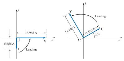
FIG. 15.12 Phasor diagrams for Examples 15.3 and 15.4.
