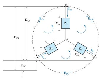
FIG. 23.36 Unbalanced, three-phase, three-wire, Y-connected load.
