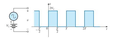
**FIG. 24.25** *Raising the base-line voltage of a square wave to zero volts.*
