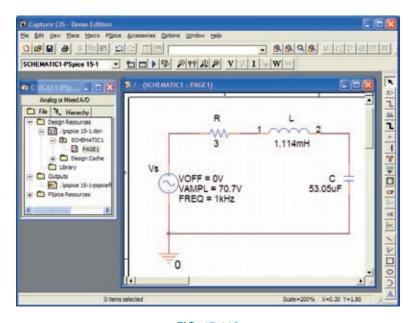
FIG. 15.116 Using PSpice to analyze a series R-L-C ac circuit.
