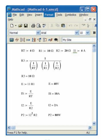
FIG. 6.25 Using Mathcad to confirm the results of Example 6.14.
