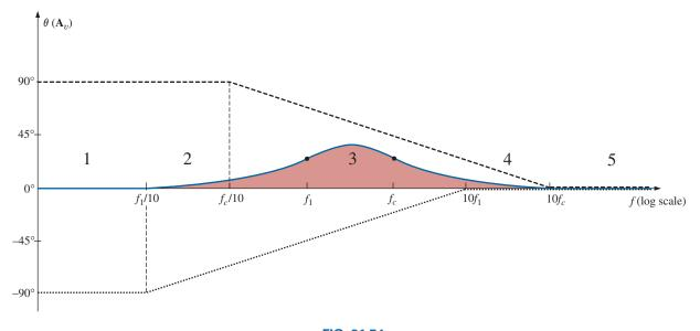
**FIG. 21.74** *Phase response for the high-pass filter in Fig. 21.68.*
