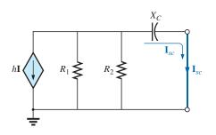
FIG. 18.49 Determining the short-circuit current for the network in Fig. 18.47.
