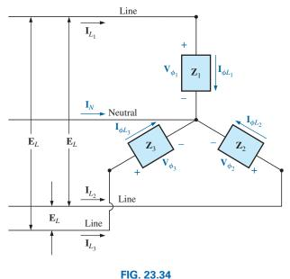
Unbalanced Y-connected load.
