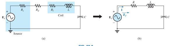
**FIG. 20.2** Series resonant circuit.
