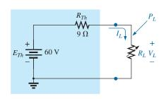
FIG. 9.79 Thévenin equivalent network to be used to validate the maximum power transfer theorem.
