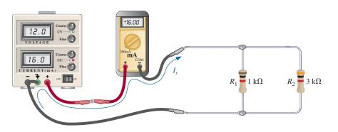
**FIG. 6.27** *Measuring the source current of a parallel network.*
