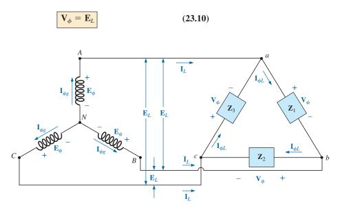
**FIG. 23.14** *Y-connected generator with a*  $\Delta$ *-connected load.*
