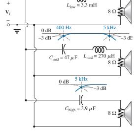
FIG. 21.83 Three-way, crossover network with 6 dB per octave.
