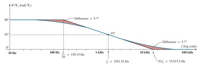
**FIG. 21.50** *Phase plot for the high-pass R-C filter.*
