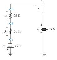
FIG. 5.61 Redrawing the circuit in Fig. 5.59 using standard dc voltage supply symbols.
