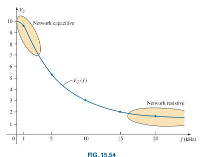
The magnitude of the voltage  $V_c$  versus frequency for the circuit in Fig. 15.47.
