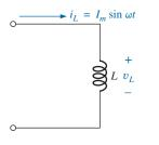
FIG. 14.8 Investigating the sinusoidal response of an inductive element.
