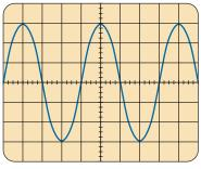
Vertical sensitivity = 50 mV/div. Horizontal sensitivity =  $10 \mu$ s/div.
