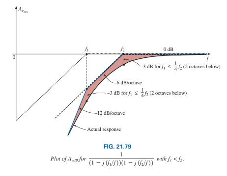
Keep in mind that if the corner frequencies of the two terms in the numerator or denominator are close but not exactly equal, the total dB drop is the algebraic sum of the contributing terms of the expansion. For instance, consider the linearized Bode plot in Fig. 21.79 with corner frequencies  $f_1$  and  $f_2$ .
