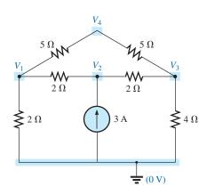
**FIG. 8.64** Defining the nodes for the network in Fig. 8.63.
