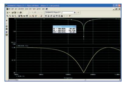
**FIG. 21.95** *dB and magnitude plot for the voltage across*  $R_L$  *of the network in Fig. 21.93.*
