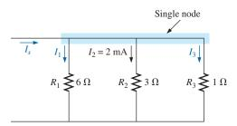
**FIG. 6.40** Parallel network for Example 6.21.
