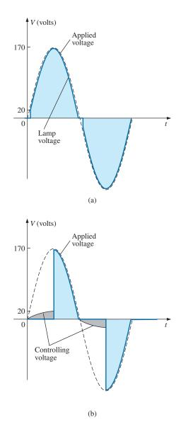
FIG. 15.113 Light dimmer: (a) with purely resistive elements; (b) half-cycle power distribution.
