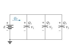
FIG. 10.68 Parallel capacitors.
