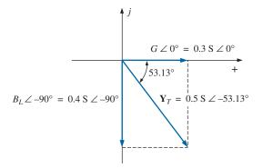
FIG. 15.70 Admittance diagram for the parallel R-L network in Fig. 15.68.
