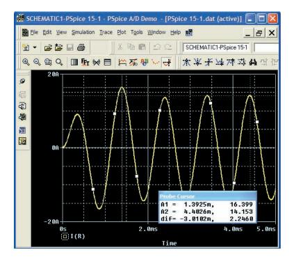
**FIG. 15.117** A plot of the current for the circuit in Fig. 15.116 showing the transition from the transient state to the steady-state response.
