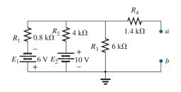
FIG. 9.49 Identifying the terminals of particular interest for the network in Fig. 9.48.
