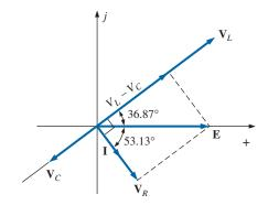
FIG. 15.38 Phasor diagram for the series R-L-C circuit in Fig. 15.35.
