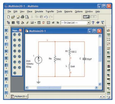
**FIG. 20.47** Using Multisim to confirm the results of Example 20.9.
