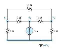
**FIG. 8.65** Reducing the number of nodes for the network in Fig. 8.63 by combining the two 5  $\Omega$  resistors.
