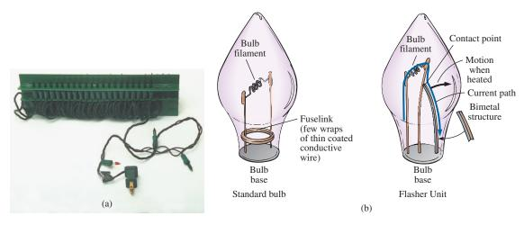
FIG. 5.78 Holiday lights: (a) 50-unit set; (b) bulb construction.
