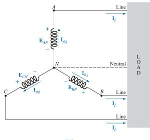
**FIG. 23.5** *Y-connected generator.*
