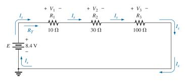
**FIG. 5.12** Schematic representation for a dc series circuit.
