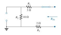
**FIG. 9.89** Determining  $R_{Th}$  for the network external to resistor  $R_L$  in Fig. 9.88.
