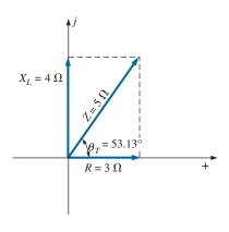
FIG. 15.28 Impedance diagram for the series R-L circuit in Fig. 15.26.
