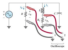
**FIG. 15.109** Determining the phase relationship between  $i_R$  and  $i_{1}$ .
