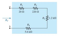
**FIG. 5.6** Series connection of resistors for Example 5.1.
