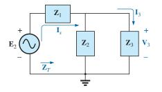
FIG. 18.15Assigning the subscripted impedances to the network<br/>in Fig. 18.14.and
