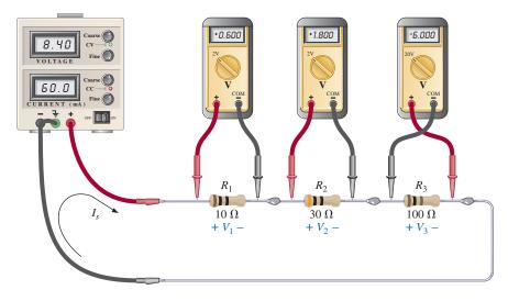
**FIG. 5.19** Using voltmeters to measure the voltages across the resistors in Fig. 5.12.
