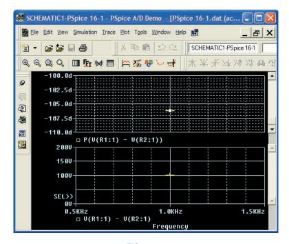
FIG. 16.33 The PSpice response for the voltage between the two points above resistors  $R_1$  and  $R_2$ .
