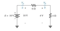
FIG. 5.51 Defining the use of single-subscript notation for voltage levels.
