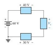
FIG. 5.30 Series configuration to be examined in Example 5.11.
