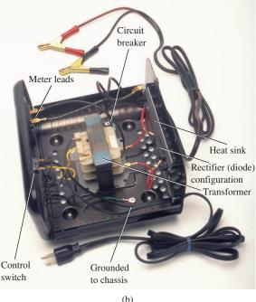
FIG. 2.32 Battery charger: (a) external appearance; (b) internal construction.
