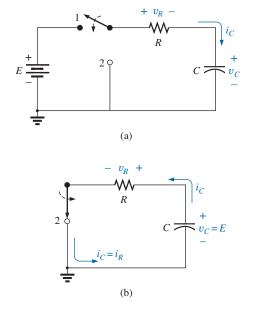
**FIG. 10.39** (a) Charging network; (b) discharging configuration.
