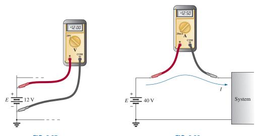
**FIG. 2.27** Voltmeter connection for an up-scale (+) reading.
