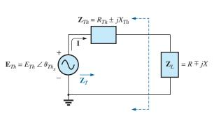
**FIG. 18.82** Conditions for maximum power transfer to  $\mathbf{Z}_{L}$ .
