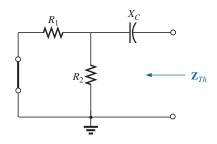
FIG. 18.42 Determining the Thévenin impedance for the network in Fig. 18.41.
