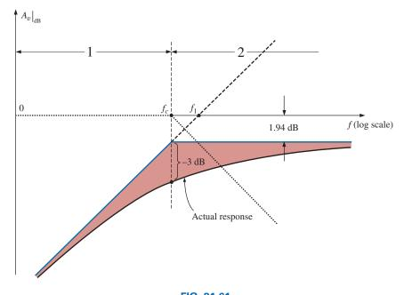
**FIG. 21.61** Plot of  $A_{v|dB}$  for the network in Fig. 21.55.
