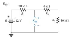
**FIG. 11.48** Determining  $E_{Th}$  for the network in Fig. 11.46.
