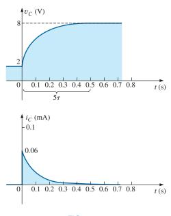
**FIG. 24.21**  $v_c$  and  $i_c$  for the network in Fig. 24.20.
