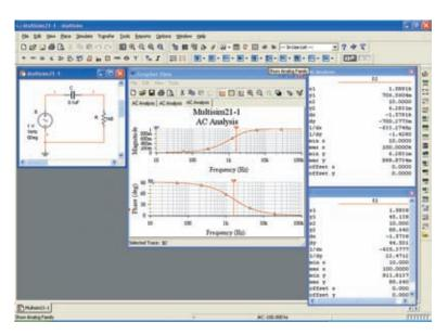
FIG. 21.96 High-pass R-C filter to be investigated using PSpice.
