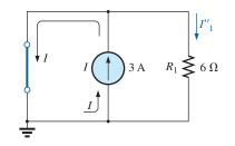
**FIG. 9.4** Determining the effect of the 3 A current source on the current  $I_1$  in Fig. 9.2.
