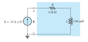
**FIG. 15.102** Series equivalent circuit for the parallel *R*-L-*C* network in Fig. 15.99 with  $\omega = 1000$  rad/s.
