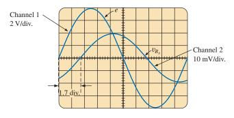
**FIG. 15.105** *e and*  $v_{R_{v}}$ , for the configuration in Fig. 15.104.
