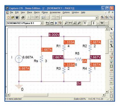
**FIG. 8.100** Applying PSpice to the bridge network in Fig. 8.72.
