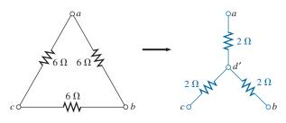
**FIG. 8.92** *Converting the*  $\Delta$  *configuration of Fig. 8.91 to a Y configuration.*
