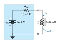
FIG. 11.52 Thévenin equivalent circuit for the network in Fig. 11.51 for  $t \ge 0$  s.
