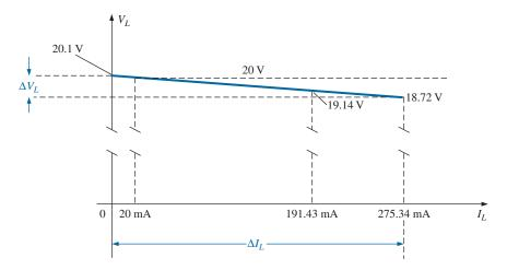
**FIG. 5.67** *Plotting*  $V_L$  versus  $I_L$  for the supply in Fig. 5.66.
