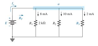
**FIG. 6.36** Parallel network for Example 6.19.
