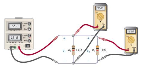
**FIG. 6.26** *Measuring the voltages of a parallel dc network.*
