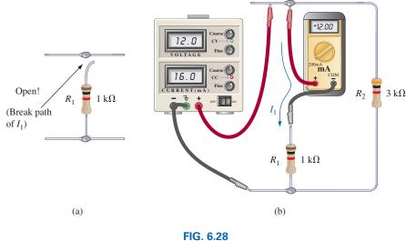
*Measuring the current through resistor*  $R_1$ .
