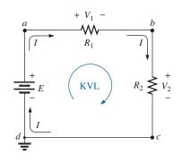
FIG. 5.26 Applying Kirchhoff's voltage law to a series dc circuit.
