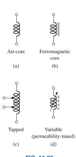
FIG. 11.20 Inductor (coil) symbols.
