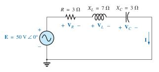
**FIG. 15.36** Applying phasor notation to the circuit in Fig. 15.35.
