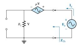
**FIG. 18.55** Determining  $\mathbf{Z}_{Th}$  using the approach  $\mathbf{Z}_{Th} = \mathbf{E}_g / \mathbf{I}_g$ .
