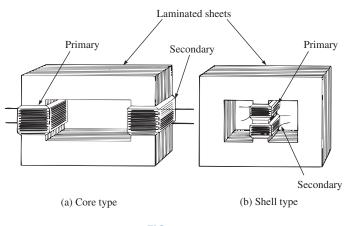
FIG. 22.37 Types of ferromagnetic core construction.
