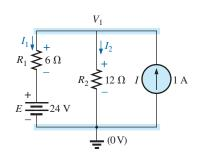
**FIG. 8.48** Applying Kirchhoff's current law to the node V<sub>1</sub>.
