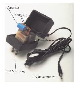
FIG. 2.35 Internal construction of the 9 V dc supply in Fig. 2.34.
