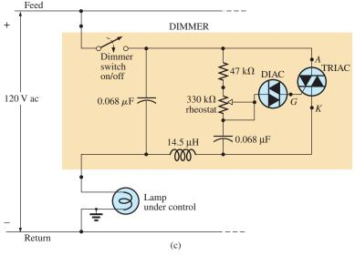
**FIG. 11.67** Dimmer control: (a) external appearance; (b) internal construction; (c) schematic.
