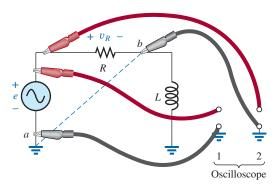
FIG. 15.108 An improper phase-measurement connection.
