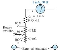
FIG. 7.52 Multirange voltmeter.
