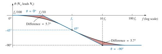
**FIG. 21.53** *Phase plot for a low-pass R-C filter.*
