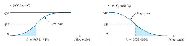
FIG. 21.27 Phase plots for a low-pass and a high-pass filter using the same elements.
