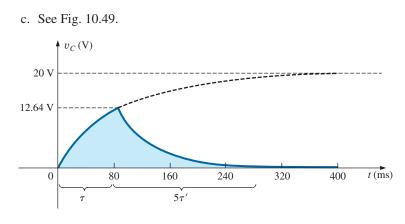
FIG. 10.49  $v_C$  for the network in Fig. 10.47.
