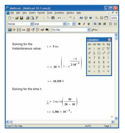
**FIG. 10.56** Applying Mathcad to the transient R-C equations.
