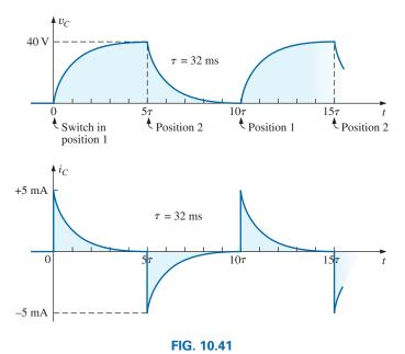
$v_C$  and  $i_C$  for the network in Fig. 10.39(a) with the values in Example 10.6.
