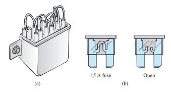
**FIG. 6.66** *Car fuses: (a) fuse link; (b) plug-in.*
