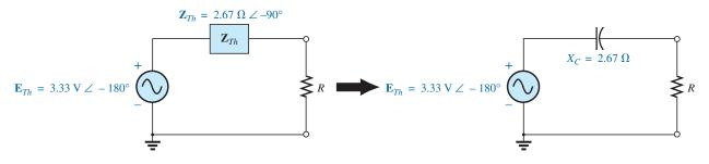
FIG. 18.28 The Thévenin equivalent circuit for the network in Fig. 18.24.
