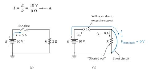
FIG. 6.52 Demonstrating the effect of a short circuit on current levels.
