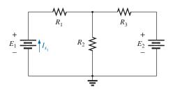
FIG. 8.19 Demonstrating the need for an approach such as branch-current analysis.
