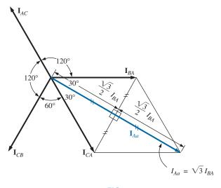
**FIG. 23.17** Determining a line current from the phase currents of a  $\Delta$ -connected, three-phase generator.
