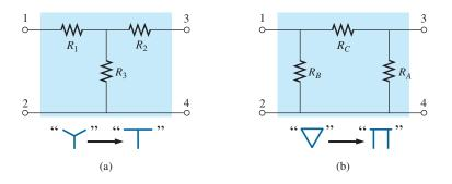
**FIG. 8.84** The relationship between the Y and T configurations and the  $\Delta$  and  $\pi$  configurations.
