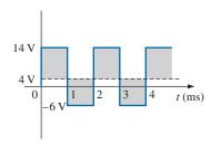
FIG. 13.43 Defining the average value for the waveform in Fig. 13.42(b).
