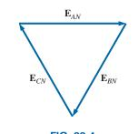
FIG. 23.4 Demonstrating that the vector sum of the phase voltages of a three-phase generator is zero.
