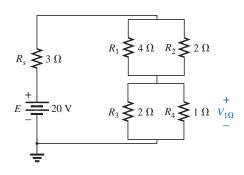
**FIG. 8.77** *Redrawing the network in Fig. 8.76.*
