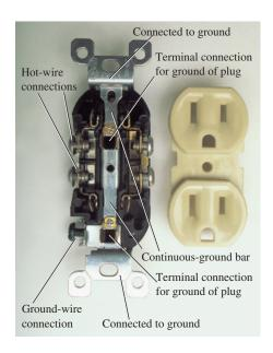
FIG. 6.68 Continuous ground connection in a duplex outlet.
