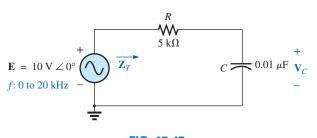
FIG. 15.47 Determining the frequency response of a series R-C circuit.
