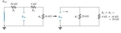
**FIG. 11.47** Determining  $R_{Th}$  for the network in Fig. 11.46.
