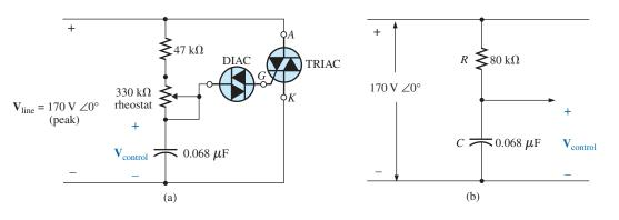
**FIG. 15.114** Light dimmer: (a) from Fig. 11.68; (b) with rheostat set at 33  $k\Omega$ .
