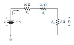
**FIG. 5.42** *Circuit in Fig. 5.41 with*  $R_2$  *and*  $R_3$  *interchanged.*
