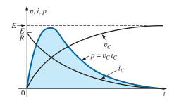
FIG. 10.76 Plotting the power to a capacitive element during the transient phase.
