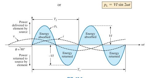
**FIG. 19.9** *The power curve for a purely inductive load.*
