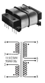
FIG. 22.38 Split bobbin, low-profile power transformer. (Courtesy of Microtran Company, Inc.)
