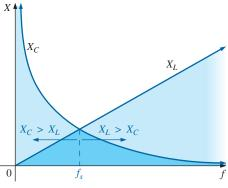
FIG. 20.11 Placing the frequency response of the inductive and capacitive reactance of a series R-L-C circuit on the same set of axes.
