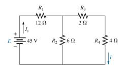
**FIG. 9.107** Finding the current I due to a source E.
