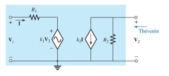
FIG. 18.57 Example 18.13: Transistor equivalent network.
