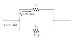
FIG. 6.45 A design-type problem for two parallel resistors (Example 6.24).
