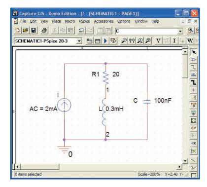
FIG. 20.44 Parallel resonant network to be analyzed using PSpice.
