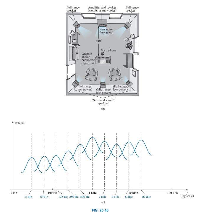
(a) Dual-channel 15-band "Constant Q" graphic equalizer (Courtesy of ARX Systems.); (b) setup; (c) frequency response.
