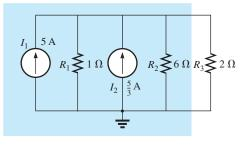
FIG. 9.98 Converting the sources in Fig. 9.97 to current sources.
