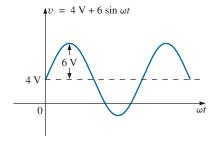
**FIG. 25.21** Wave pattern generated by the source in Fig. 25.20.
