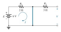
**FIG. 6.60** Network in Fig. 6.59 with  $R_2$  replaced by a jumper.
