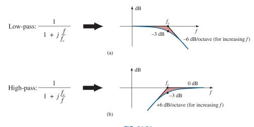
**FIG. 21.54** *dB response of (a) low-pass filter and (b) high-pass filter.*
