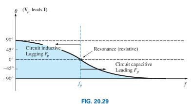
Phase plot for the parallel resonant circuit.
