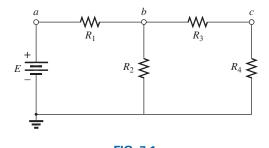
FIG. 7.1 Series-parallel dc network.
