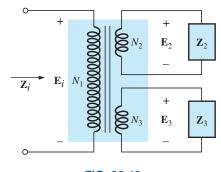
FIG. 22.43 Ideal transformer with multiple loads.
