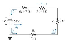
**FIG. 5.16** Series circuit to be analyzed in Example 5.5.
