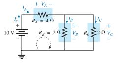
**FIG. 7.11** *Reduced equivalent of Fig. 7.10.*
