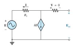
FIG. 18.79 Determining  $\mathbf{E}_{oc}$  for the network in Fig. 18.77.
