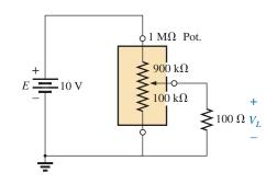
**FIG. 7.44** Loaded potentiometer with  $R_L \ll R_T$ .
