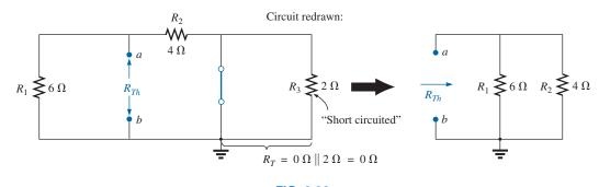
**FIG. 9.39** Determining  $R_{Th}$  for the network in Fig. 9.38.
