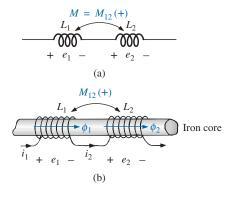
**FIG. 22.25** *Mutually coupled coils connected in series.*
