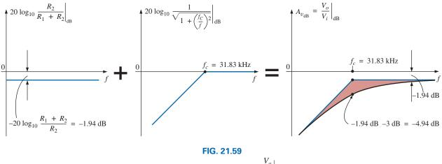
Obtaining a dB plot of  $A_{v_{dB}} = \frac{V_o}{V_i}\Big|_{dB}$ .
