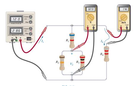
**FIG. 7.7** Inserting an ammeter and a voltmeter to measure  $I_4$  and  $V_2$ , respectively.
