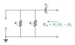
**FIG. 18.48** Determining the Thévenin impedance for the network in Fig. 18.47.
