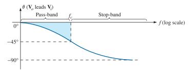
**FIG. 21.13** Angle by which  $V_o$  leads  $V_i$ .
