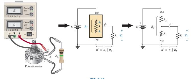
FIG. 7.43 Loaded potentiometer.
