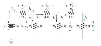
FIG. 7.37 An alternative approach for ladder networks.
