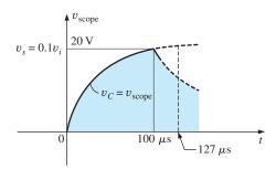
**FIG. 24.40** The scope pattern for the conditions in Fig. 24.38 with  $v_i = 200$  V peak.
