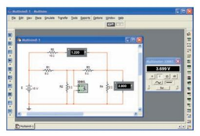
**FIG. 8.101** Using Multisim to verify the results in Example 8.18.
