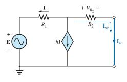
FIG. 18.78 Determining  $I_{sc}$  for the network in Fig. 18.77.
