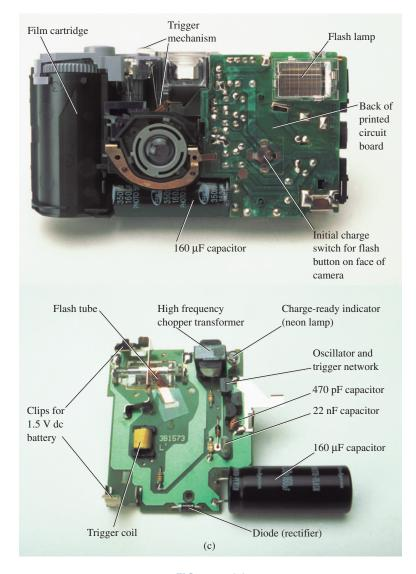
FIG. 10.78(c) Flash camera: internal construction.
