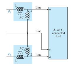
FIG. 23.30 *Two-wattmeter method for a*  $\Delta$ *- or a* Y-connected load.
