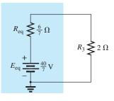
FIG. 9.100 Converting the current source in Fig. 9.99 to a voltage source.
