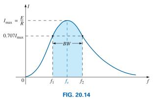
I versus frequency for the series resonant circuit.
