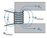
**FIG. 22.16** *Identifying the leakage flux of the primary.*
