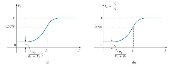
**FIG. 21.70** *High-pass filter with limited attenuation.*
