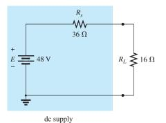
**FIG. 9.87** *dc supply with a fixed 16*  $\Omega$  *load (Example 9.16).*
