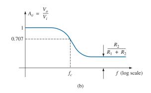
FIG. 21.63 Low-pass filter with limited attenuation.
