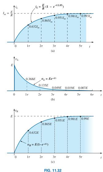
$i_L$ ,  $v_L$ , and  $v_R$  for the circuit in Fig. 11.31 following the closing of the switch.
