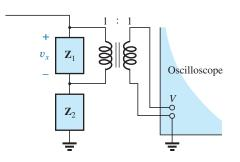
FIG. 22.13 Correcting the situation of Fig. 22.12 using an isolation transformer.
