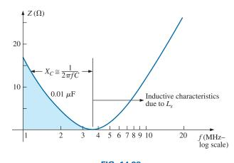
**FIG. 14.28** Impedance characteristics of a 0.01  $\mu$ F metalized film capacitor versus frequency.
