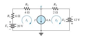
FIG. 8.34 Defining the mesh currents for the network in Fig. 8.33.
