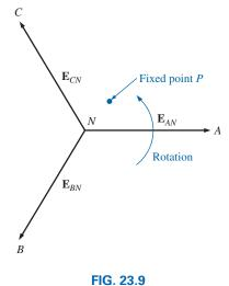
Determining the phase sequence from the phase voltages of a three-phase generator.
