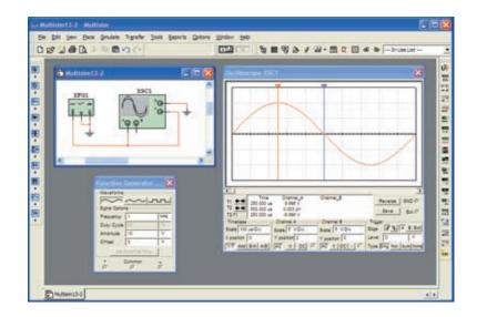
FIG. 13.79 Using the function generator to place a sinusoidal ac voltage waveform on the screen of the oscilloscope.
