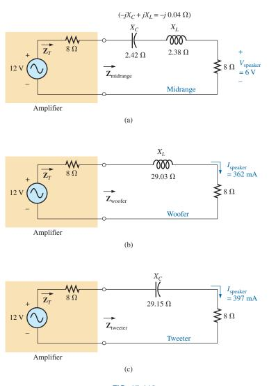
**FIG. 15.112** Crossover network: (a) mid-range speaker at 1.4 kHz; (b) woofer at 1.4 kHz; (c) tweeter.
