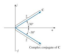
FIG. 14.54 Defining the complex conjugate of a complex number in polar form.
