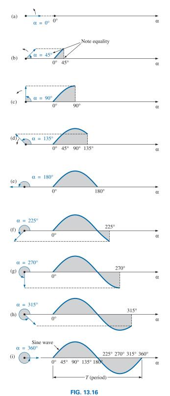
*Generating a sinusoidal waveform through the vertical projection of a rotating vector.*
