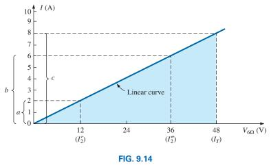
Plotting I versus V for the 6  $\Omega$  resistor.
