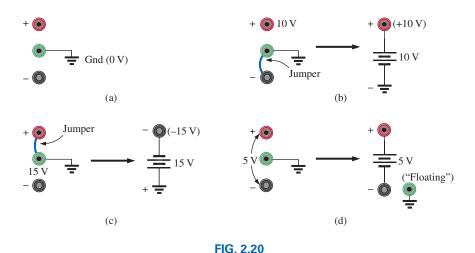
dc laboratory supply: (a) available terminals; (b) positive voltage with respect to (w.r.t.) ground; (c) negative voltage w.r.t. ground; (d) floating supply.
