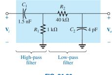
**FIG. 21.30** Pass-band filter.
