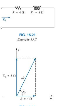
FIG. 15.22 Impedance diagram for Example 15.7.
