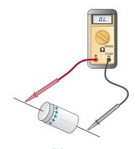
**FIG. 10.25** Checking the dielectric of an electrolytic capacitor.
