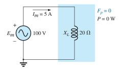
**FIG. 14.34** *Purely inductive load with*  $F_p = 0$ .
