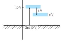
**FIG. 5.57** Determining  $V_b$  using the defined voltage levels.
