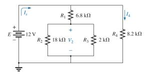
FIG. 7.5 Series-parallel network for Example 7.2.
