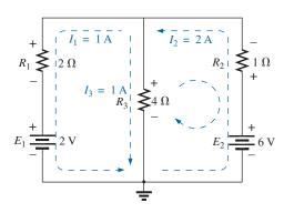
FIG. 8.27 Reviewing the results of the analysis of the network in Fig. 8.22.
