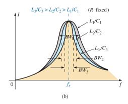
FIG. 20.15 Effect of R, L, and C on the selectivity curve for the series resonant circuit.
