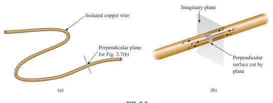
FIG. 2.7 There is motion of free carriers in an isolated piece of copper wire, but the flow of charge fails to have a particular direction.
