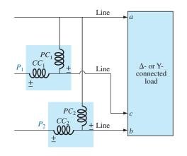
FIG. 23.31 Alternative hookup for the two-wattmeter method.
