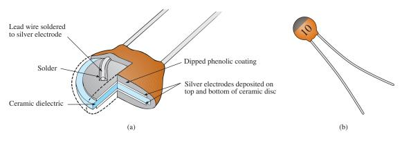
**FIG. 10.16** *Ceramic (disc) capacitor: (a) construction; (b) appearance.*
