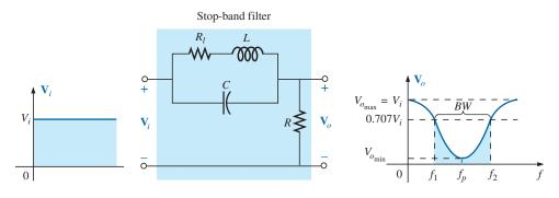
**FIG. 21.42** *Stop-band filter using a parallel resonant network.*
