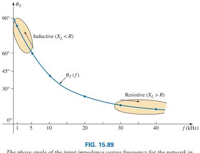
The phase angle of the input impedance versus frequency for the network in Fig. 15.86.
