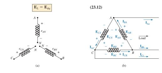
**FIG. 23.16**  $\Delta$ *-connected generator.*
