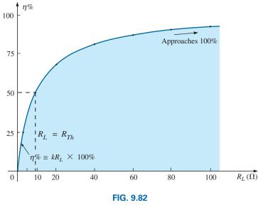
Efficiency of operation versus increasing values of  $R_L$ .
