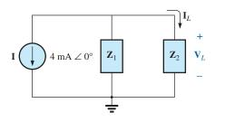
FIG. 16.11 Network in Fig. 16.10 following the assignment of the block impedances.
