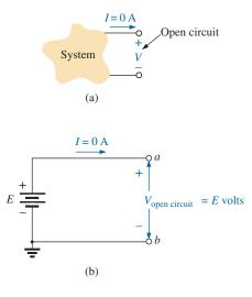
**FIG. 6.49** *Defining an open circuit.*
