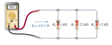
FIG. 6.17 Using an ohmmeter to measure the total resistance of a parallel network.
