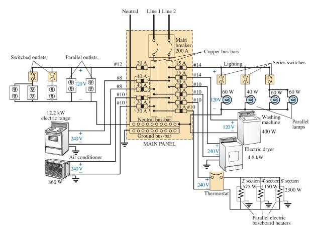
**FIG. 15.110** *Home wiring diagram.*  note the series connection of switches to lights in the upper-right corner but the parallel connection of lights and outlets. Due to high current demand, the air conditioner, heaters, and electric stove have 30 A breakers. Keep in mind that the total current does not equal the product of the two (or 60 A) since each breaker is in a line and the same current will flow through each breaker.
