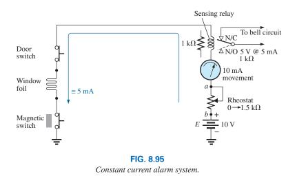
If any of the sensors open, the current through the entire circuit drops to zero, the coil of the relay releases the plunger, and contact is made with the N/C position of the relay. This action completes the circuit for the bell circuit, and the alarm sounds. For the future, keep in mind that
