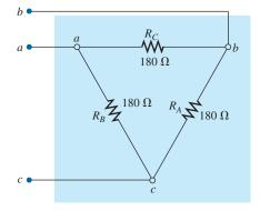
**FIG. 8.88** *The*  $\Delta$  *equivalent for the Y in Fig.* 8.87.
