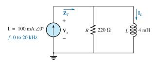
FIG. 15.86 Determining the frequency response of a parallel R-L network.
