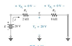
FIG. 6.63 A malfunctioning network.
