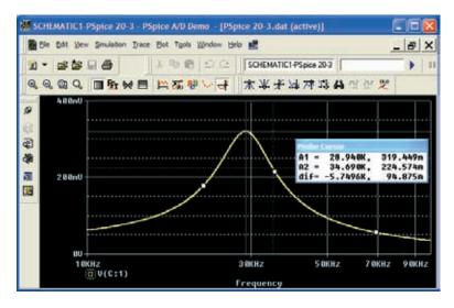
**FIG. 20.45** *Resonance curve for the voltage across the capacitor in Fig. 20.44.*
