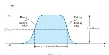
FIG. 24.2 Actual pulse waveform.
