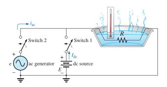
FIG. 13.57 An experimental setup to establish a relationship between dc and ac quantities.
