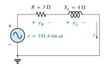
FIG. 15.26 Series R-L circuit.
