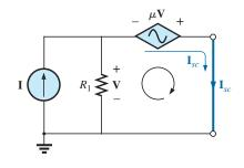
**FIG. 18.53** Determining  $I_{sc}$  for the network in Fig. 18.51.
