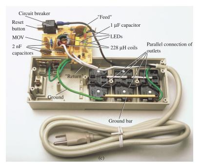
FIG. 10.79(c) Internal construction.
