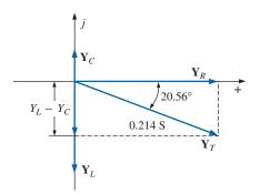
**FIG. 15.65** Admittance diagram for the network in Fig. 15.63.
