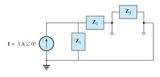
**FIG. 18.68** *Assigning the subscripted impedances to the network in Fig. 18.67.*
