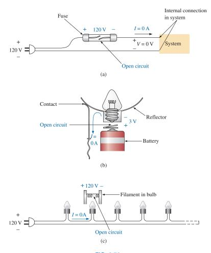
FIG. 6.50 Examples of open circuits.
