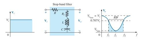
**FIG. 21.41** Stop-band filter using a series resonant circuit.
