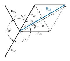
**FIG. 23.7** Determining a line voltage for a three-phase generator.
