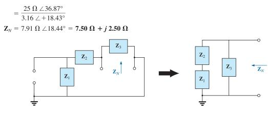
**FIG. 18.69** *Finding the Norton impedance for the network in Fig. 18.67.*
