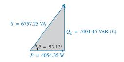
FIG. 19.30 Initial power triangle for the load in Example 19.7.
