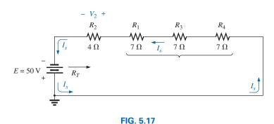
Circuit in Fig. 5.16 redrawn to permit the use of Eq. (5.2).
