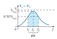
**FIG. 21.34** Parallel resonant pass-band filter.
