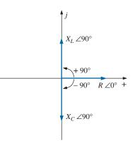
FIG. 15.19 Impedance diagram.
