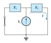
FIG. 18.8 Determining the effect of the current source I<sub>1</sub> on the current I of the network in Fig. 18.6.
