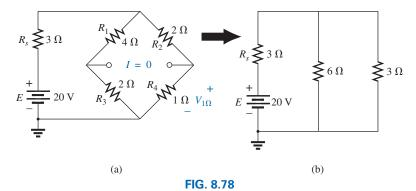
Substituting the open-circuit equivalent for the balance arm of a balanced bridge.
