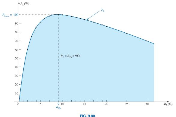
$P_L$  versus  $R_L$  for the network in Fig. 9.79.
