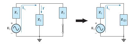
FIG. 18.3 Determining the effect of the voltage source  $\mathbf{E}_1$  on the current I of the network in Fig. 18.1.
