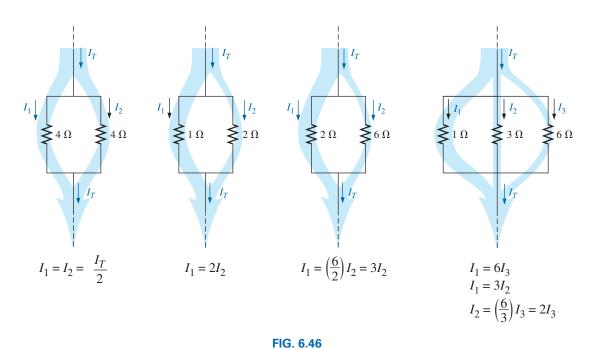
Demonstrating how current divides through equal and unequal parallel resistors.
