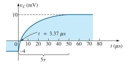
**FIG. 24.23**  $v_C$  for the network in Fig. 24.22.
