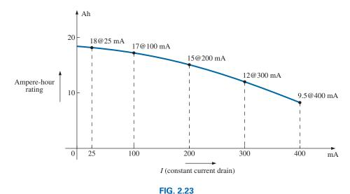
Ampere-hour rating (capacity) versus drain current for an Energizer® D cell.
