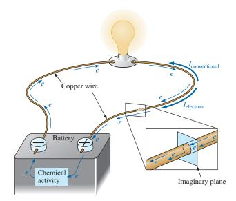
**FIG. 2.9** *Basic electric circuit.*
