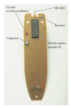
FIG. 24.44 Back side of TV remote in Fig. 24.43.
