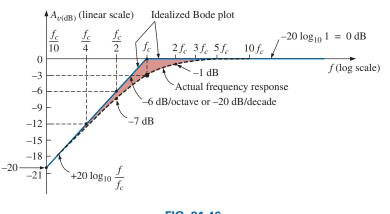
FIG. 21.46 Idealized Bode plot for the low-frequency region.
