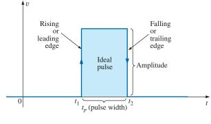
FIG. 24.1 Ideal pulse waveform.
