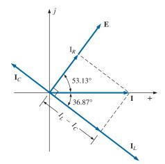
*Phasor diagram:* The phasor diagram in Fig. 15.80 indicates that the impressed voltage **E** is in phase with the current  $I_R$  through the resistor, leads the current  $I_L$  through the inductor by 90°, and lags the current  $I_C$  of the capacitor by 90°. *Time domain:*
