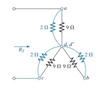
**FIG. 8.93** Substituting the Y configuration for the converted  $\Delta$  into the network in Fig. 8.91.
