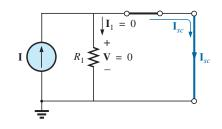
**FIG. 18.54** Substituting  $\mathbf{V} = 0$  into the network in Fig. 18.53.
