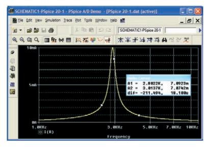
**FIG. 20.43** *Resonance curve for the current of the circuit in Fig. 20.42.*
