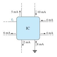
**FIG. 6.38** Integrated circuit for Example 6.20.
