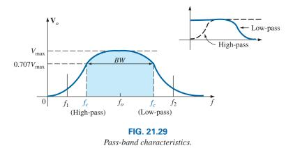
The network in Example 21.7 generates the characteristics of Fig. 21.29. However, for a circuit such as the one shown in Fig. 21.30, there is a loading between stages at each frequency that affects the level of  $\mathbf{V}_o$ . Through proper design, the level of  $\mathbf{V}_o$  may be very near the level of  $\mathbf{V}_i$
