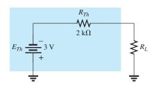
FIG. 9.53 Substituting the Thévenin equivalent circuit for the network external to the resistor  $R_L$  in Fig. 9.48.
