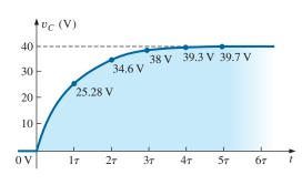
**FIG. 10.36**  $v_c$  versus time for the charging network in Fig. 10.35.
