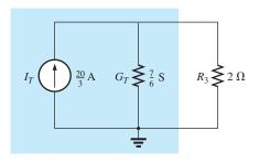
**FIG. 9.99** Reducing the current sources in Fig. 9.98 to a single source.
