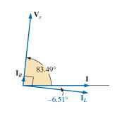
FIG. 15.92 The phasor diagram for the parallel R-L network in Fig. 15.86 at f = 1 kHz.
