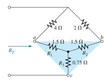
**FIG. 8.90** Substituting the Y equivalent for the bottom  $\Delta$  in Fig. 8.89.
