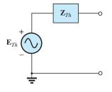
FIG. 18.23 Thévenin equivalent circuit for ac networks.
