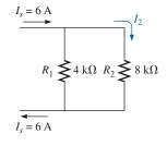
FIG. 6.44 Using the current divider rule to determine current  $I_2$ in Example 6.23.
