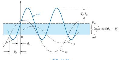
FIG. 14.32 Defining the average power for a sinusoidal ac network.
