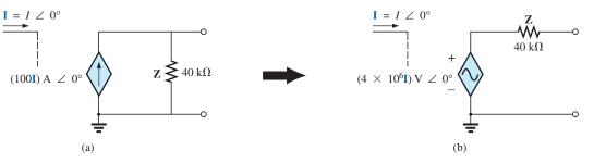
FIG. 17.9 Source conversion with a current-controlled current source.
