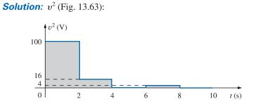
**FIG. 13.63** *The squared waveform of Fig. 13.62.*
