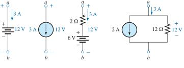
**FIG. 9.103** Equivalent branches for the branch a-b in Fig. 9.102.
