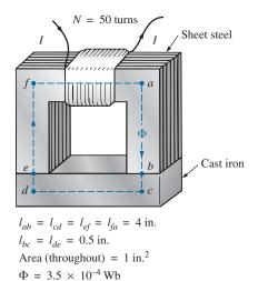
FIG. 12.14 Electromagnet for Example 12.2.
