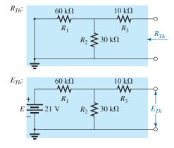
FIG. 10.58 Applying Thévenin's theorem to the network in Fig. 10.57.
