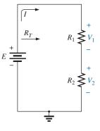
**FIG. 5.36** *Developing the voltage divider rule.*
