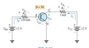
**FIG. 7.59** *dc bias levels of a transistor amplifier.*
