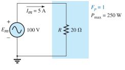
**FIG. 14.33** *Purely resistive load with*  $F_n = 1$ *.*
