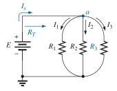
FIG. 6.37 Redrawn network in Fig. 6.36.
