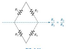
FIG. 8.80 A visual approach to remembering the balance condition.
