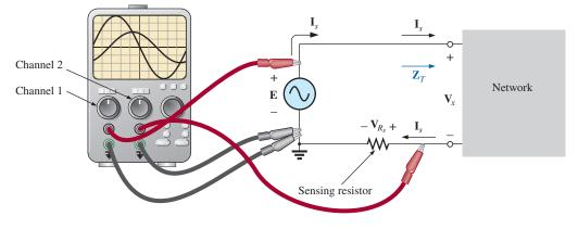
**FIG. 15.104** Using an oscilloscope to measure  $Z_T$  and  $\theta_T$ .
