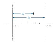
FIG. 21.3 Finding a value on a log plot.
