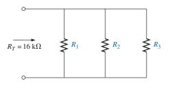
FIG. 6.16 Parallel network for Example 6.11.
