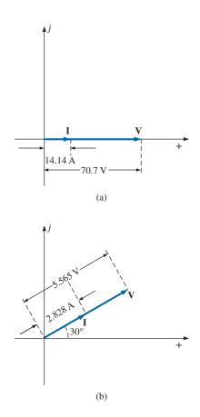
FIG. 15.6 Phasor diagrams for Examples 15.1 and 15.2.
