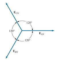
FIG. 23.3 Phasor diagram for the phase voltages of a three-phase generator.
