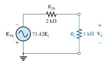
**FIG. 18.38** The Thévenin equivalent circuit for the network in Fig. 18.35.
