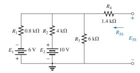
FIG. 9.110 Network to which PSpice is to be applied to determine  $E_{Th}$  and  $R_{Th}$ .
