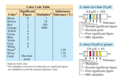
Cylindrical molded choke coils are marked with five colored bands. A wide silver band, located at one end of the coil, identifies military radio-frequency coils. The next three bands indicate the inductance in microhenries, and the fourth band is the tolerance.
