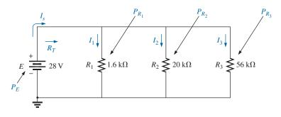
**FIG. 6.30** Parallel network for Example 6.15.
