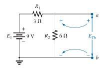
**FIG. 9.29** Determining  $E_{Th}$  for the network in Fig. 9.27.
