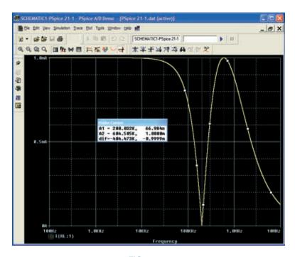
**FIG. 21.94** Magnitude plot versus frequency for the voltage across  $R_L$  of the network in Fig. 21.93.
