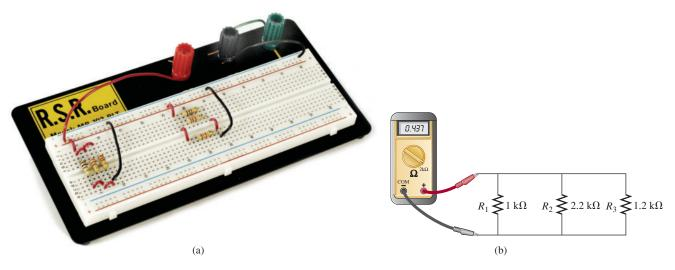
**FIG. 6.64** Using a protoboard to set up the circuit in Fig. 6.17.
