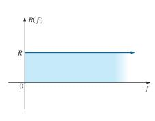
FIG. 20.8 Resistance versus frequency.
