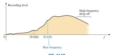
**FIG. 21.90** *Noise reduction in a tape recorder.*
