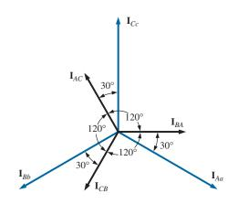
FIG. 23.18 The phasor diagram of the currents of a three-phase,  $\Delta$ -connected generator.
