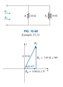
**FIG. 15.61** Impedance diagram for the network in Fig. 15.60.
