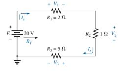
**FIG. 5.15** Series circuit to be investigated in Example 5.4.
