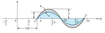
**FIG. 13.35** *Example 13.12(e):* v and i are in phase.
