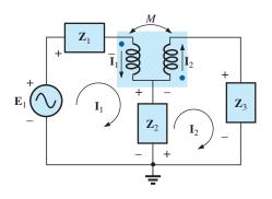
FIG. 22.45 Applying mesh analysis to magnetically coupled coils.
