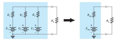
**FIG. 9.91** Demonstrating the effect of applying Millman's theorem.
