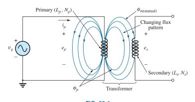
**FIG. 22.1** *Defining the components of a transformer.*
