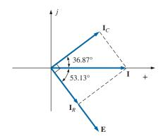
FIG. 15.75 Phasor diagram for the parallel R-C network in Fig. 15.74.
