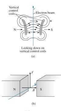
FIG. 11.72 Deflection coils: (a) vertical control; (b) right-handrule (RHR) for electron flow.
