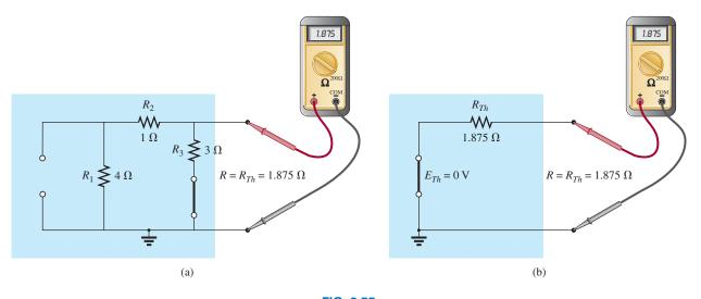
**FIG. 9.55** Measuring  $R_{Th}$  with an ohmmeter: (a) actual network; (b) Thévenin equivalent.
