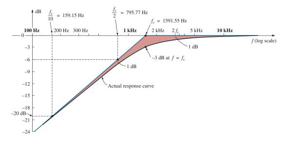
**FIG. 21.49** Frequency response for the high-pass filter in Fig. 21.48.
