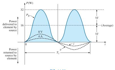
**FIG. 14.30** *Power versus time for a purely resistive load.*
