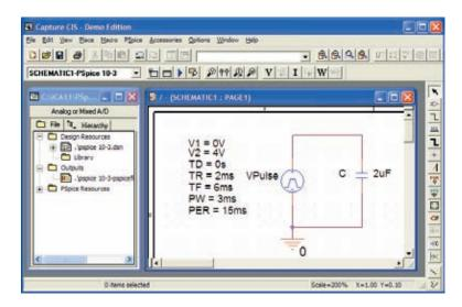
FIG. 10.85 Using PSpice to verify the results in Example 10.14.
