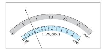
**FIG. 21.6** Defining the relationship between a dB scale referenced to 1 mW, 600  $\Omega$  and a 3 V rms voltage scale.
