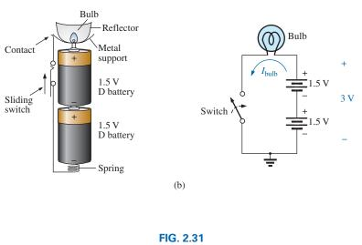
(a) Eveready<sup>®</sup> D cell flashlight; (b) electrical schematic of flashlight of part (a);
