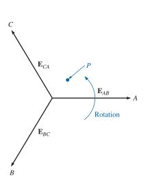
FIG. 23.10 Determining the phase sequence from the line voltages of a three-phase generator.
