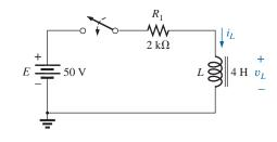
FIG. 11.36 Series R-L circuit for Example 11.3.
