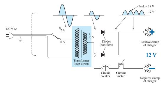
FIG. 2.33 Electrical schematic for the battery charger of Fig. 2.32.
