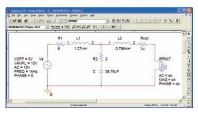
**FIG. 18.99** Using PSpice to determine the short-circuit current.
