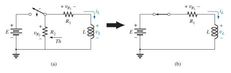
**FIG. 11.42** *Initiating the storage phase for an inductor by closing the switch.*
