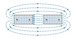
**FIG. 11.2** Flux distribution for two adjacent, opposite poles.
