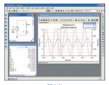
FIG. 14.81 Using Multisim to review the response of an inductive element to a sinusoidal ac signal.
