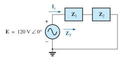
FIG. 16.2 Network in Fig. 16.1 after assigning the block impedances.
