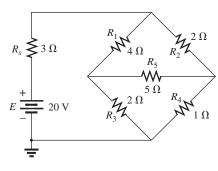
**FIG. 8.70** *Standard bridge configuration.*
