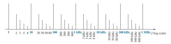
FIG. 21.2 Frequency log scale.
