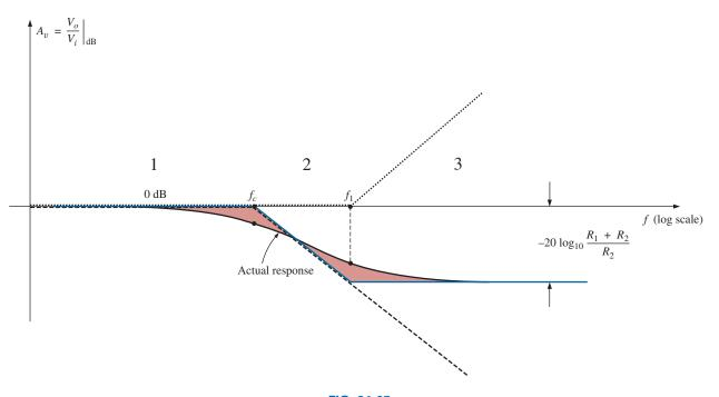
**FIG. 21.65**  $A_{v_{dB}}$  versus frequency for the low-pass filter with limited attenuation of Fig. 21.62.
