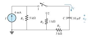
**FIG. 10.46** *Network to be analyzed in Example 10.9.*
