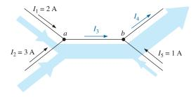
**FIG. 6.33** *Two-node configuration for Example 6.16.*
