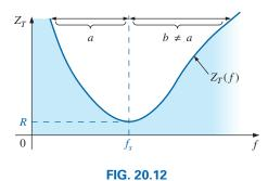
$Z_T$  versus frequency for the series resonant circuit.
