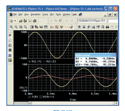
**FIG. 15.118** A plot of the steady-state response (t > 3 ms) for  $v_L$ ,  $v_s$ , and i for the circuit in Fig. 15.116.
