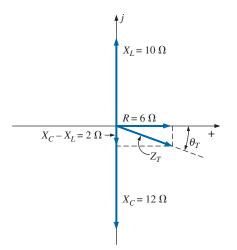
**FIG. 15.24** *Impedance diagram for Example 15.8.*
