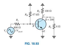
ac equivalent of the transistor network in Fig. 18.91.
