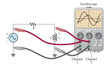
**FIG. 15.106** Determining the phase relationship between e and  $v_L$ .
