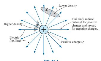
**FIG. 10.1** Flux distribution from an isolated positive charge.
