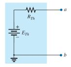
**FIG. 9.23** *Thévenin equivalent circuit.*
