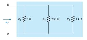
FIG. 6.5 Parallel resistors for Example 6.2.
