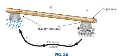
Motion of negatively charged electrons in a copper wire when placed across battery terminals with a difference in potential of volts (V).
