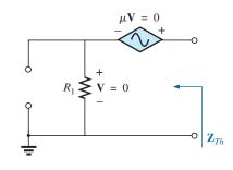
FIG. 18.52 Determining  $\mathbf{Z}_{Th}$  incorrectly.
