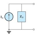
**FIG. 18.60** *The Norton equivalent circuit for ac networks.*
