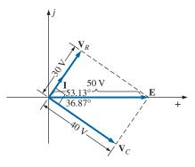
FIG. 15.33 Phasor diagram for the series R-C circuit in Fig. 15.30.
