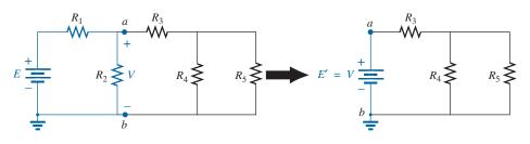
**FIG. 9.104** Demonstrating the effect of knowing a voltage at some point in a complex network.
