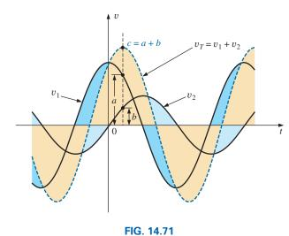
Adding two sinusoidal waveforms on a point-by-point basis.
