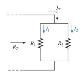
FIG. 6.43 Deriving the current divider rule for the special case of only two parallel resistors.
