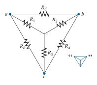
**FIG. 8.82** Introducing the concept of  $\Delta$ -Y or Y- $\Delta$  conversions.
