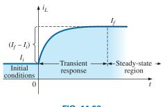
**FIG. 11.38** Defining the three phases of a transient waveform.
