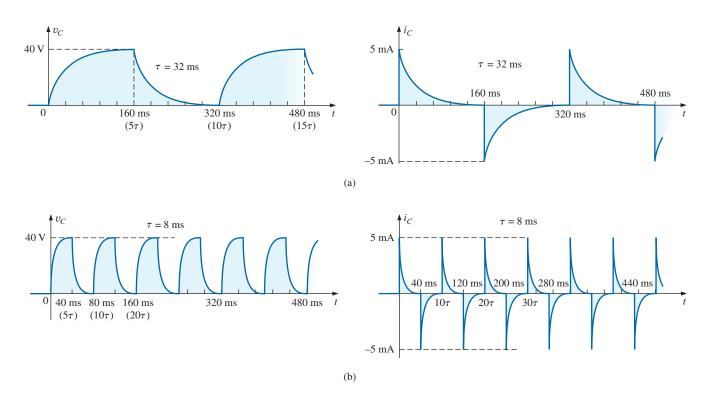
**FIG. 10.42** *Plotting*  $v_c$  *and*  $i_c$  *versus time in ms: (a)*  $\tau = 32$  *ms; (b)*  $\tau = 8$  *ms.*
