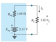
FIG. 9.96 The result of applying Millman's theorem to the network in Fig. 9.95.
