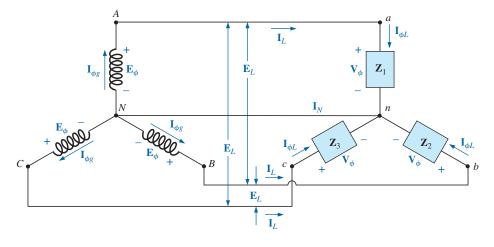
FIG. 23.12 Y-connected generator with a Y-connected load.
