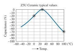
FIG. 10.22 Variation of capacitor value with temperature.
