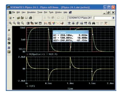
**FIG. 24.49** Plot of  $v_{pulse}$ ,  $v_C$ , and  $i_C$  for the circuit in Fig. 24.47.
