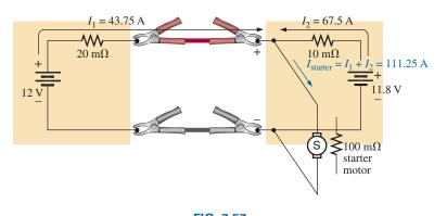
**FIG. 7.57** *Current levels at starting.*
