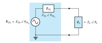
**FIG. 18.81** Defining the conditions for maximum power transfer to a load.
