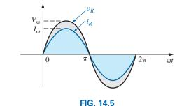
The voltage and current of a resistive element are in phase.
