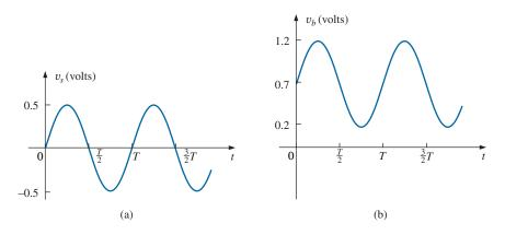
**FIG. 18.96** Applied signal: (a) at the source; (b) at the base of the transistor.
