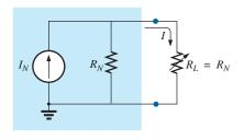
FIG. 9.84 Defining the conditions for maximum power to a load using the Norton equivalent circuit.
