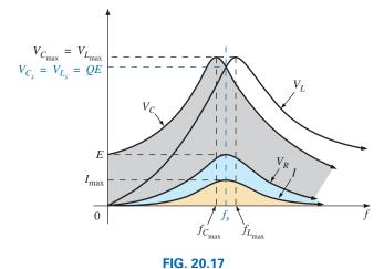
$V_R$ ,  $V_L$ ,  $V_C$ , and I versus frequency for a series resonant circuit.
