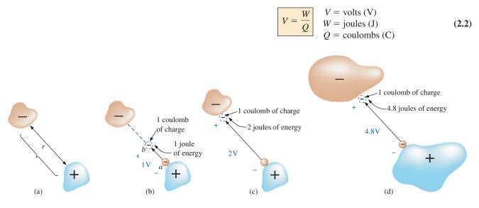
FIG. 2.5 Defining the voltage between two points.
