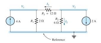
**FIG. 8.56** Applying Kirchhoff's current law to the node V<sub>2</sub>.
