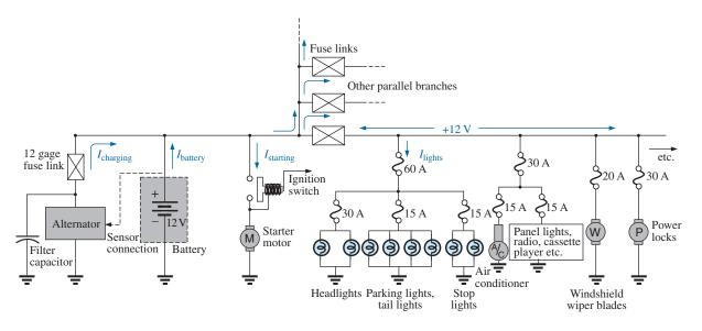
FIG. 6.65 Expanded view of an automobile's electrical system.
