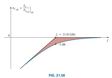
dB plot for  $A'_{v}$  for the high-pass filter in Fig. 21.55.
