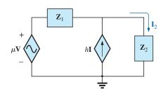
FIG. 18.19 Assigning the subscripted impedances to the network in Fig. 18.18.
