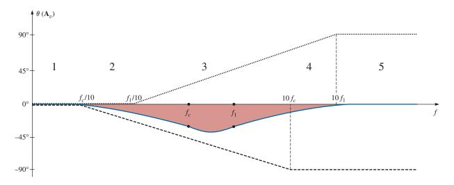
**FIG. 21.67** *Phase angle for the low-pass filter in Fig. 21.62.*
