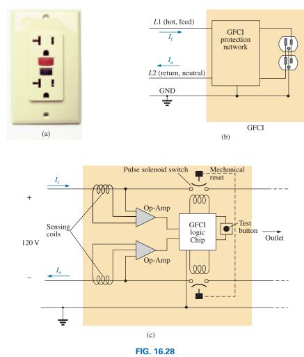
GFCI outlet: (a) wall-mounted appearance; (b) basic operation; (c) schematic.
