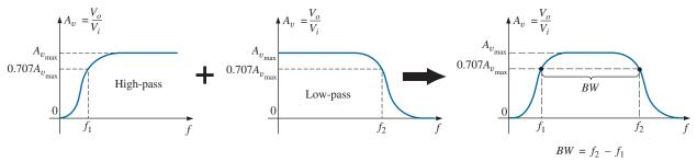
**FIG. 21.80** Finding the overall gain versus frequency for Example 21.12.
