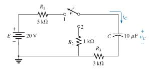
**FIG. 10.47** *The charging phase for the network in Fig. 10.46.*
