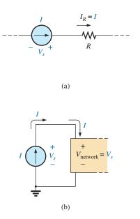
FIG. 8.1 Introducing the current source symbol.
