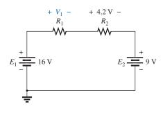
FIG. 5.27 Series circuit to be examined in Example 5.8.
