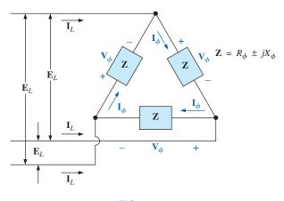
**FIG. 23.24**  $\Delta$ -connected balanced load.
