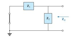
FIG. 18.64 Determining the Norton impedance for the network in Fig. 18.62.
