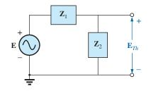
FIG. 18.27 Determining the open-circuit Thévenin voltage for the network in Fig. 18.24.
