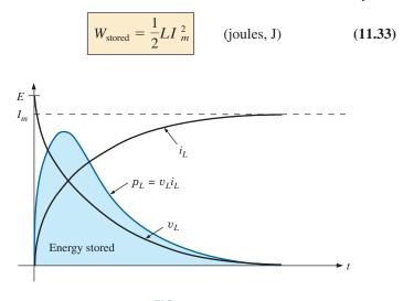
**FIG. 11.65** *The power curve for an inductive element under transient conditions.*
