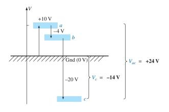
**FIG. 5.58** *Review of the potential levels for the circuit in Fig. 5.56.*
