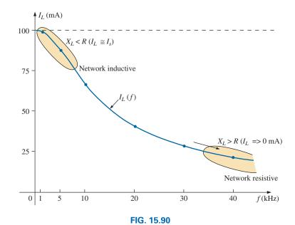
The magnitude of the current  $I_L$  versus frequency for the parallel R-L network in Fig. 15.86.
