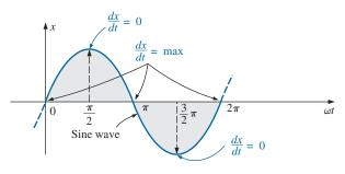
**FIG. 14.1** *Defining those points in a sinusoidal waveform that have maximum and minimum derivatives.*
