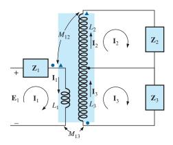
FIG. 22.46 Applying mesh analysis to a network with two magnetically coupled coils.
