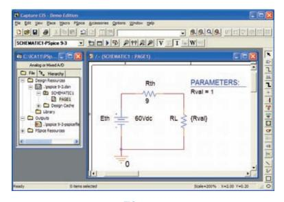
**FIG. 9.113** Using PSpice to plot the power to  $R_L$  for a range of values for  $R_L$ .
