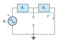
FIG. 18.9 Determining the effect of the voltage source  $\mathbf{E}_1$  on the current I of the network in Fig. 18.6.
