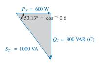
FIG. 19.22 Power triangle for Example 19.3.
