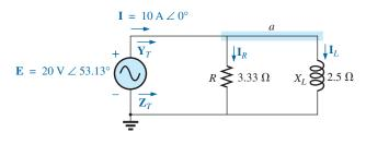
**FIG. 15.69** Applying phasor notation to the network in Fig. 15.68.
