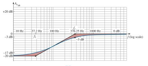
FIG. 21.76  $A_{v_{dB}}$  versus frequency for the filter in Fig. 21.75.
