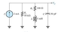
**FIG. 20.36** Equivalent network for the transistor configuration in Fig. 20.35.
