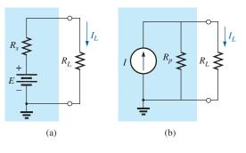
FIG. 8.5 Practical sources: (a) voltage; (b) current.
