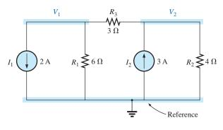
**FIG. 8.60** *Defining the nodes for the network in Fig. 8.59.*
