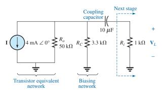
**FIG. 16.10** *Basic transistor amplifier.*
