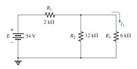
**FIG. 7.3** Series-parallel network for Example 7.1.
