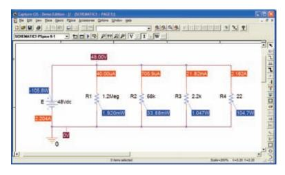
**FIG. 6.70** Applying PSpice to a parallel network.
