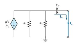
FIG. 18.44 Converting the voltage source in Fig. 18.43 to a current source.
