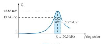
FIG. 21.36 Pass-band response for the network.
