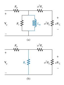
FIG. 22.22 (a) Low-frequency reflected equivalent circuit; (b) mid-frequency reflected circuit.
