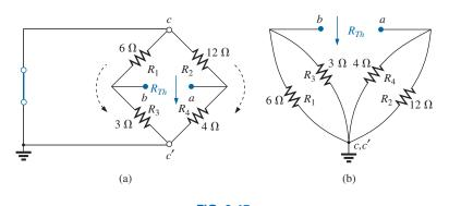
**FIG. 9.45** Solving for  $R_{Th}$  for the network in Fig. 9.44.
