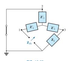
FIG. 18.87 Substituting the Y equivalent for the upper  $\Delta$ configuration in Fig. 18.86.
