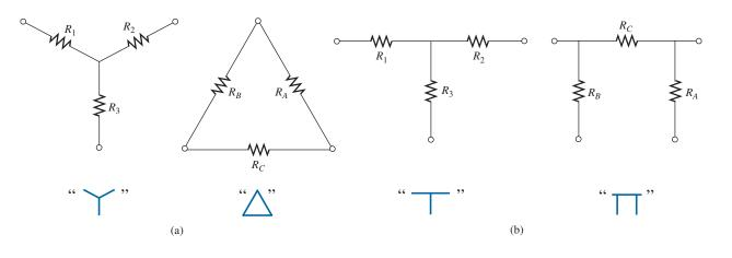
**FIG. 8.81** *The* Y(T) *and*  $\Delta(\pi)$  *configurations.*
