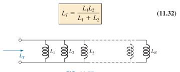
**FIG. 11.57** *Inductors in parallel.*
