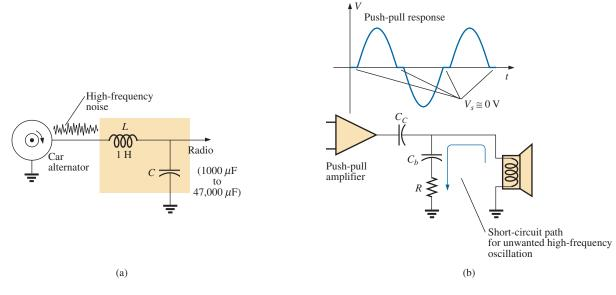
**FIG. 21.91** Noise generation: (a) due to a car alternator; (b) from a push-pull amplifier.
