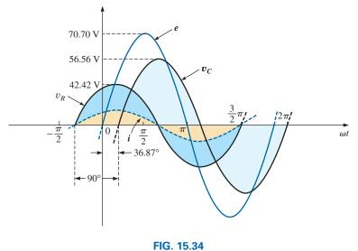
Waveforms for the series R-C circuit in Fig. 15.30.
