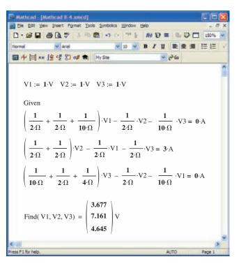
FIG. 8.66 Using Mathcad to verify the mathematical calculations of Example 8.25.
