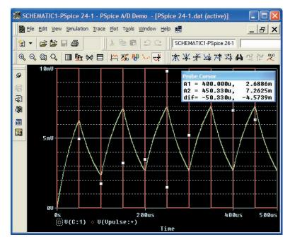
**FIG. 24.50** *Plot of*  $v_c$  *for the circuit in Fig.* 24.47 *with*  $t_p = \tau = T/2$ .
