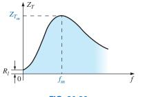
**FIG. 20.26**  $Z_T$  versus frequency for the parallel resonant circuit.
