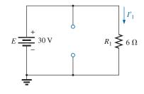
FIG. 9.3 Determining the effect of the 30 V supply on the current I<sub>1</sub> in Fig. 9.2.
