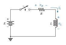
FIG. 11.31 Basic R-L transient network.
