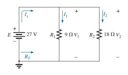
FIG. 6.22 Parallel network for Example 6.12.
