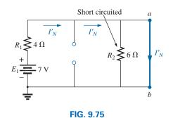
Determining the contribution to  $I_N$  from the voltage source  $E_1$ .
