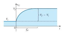
**FIG. 24.18** Defining the parameters of Eq. (24.6).
