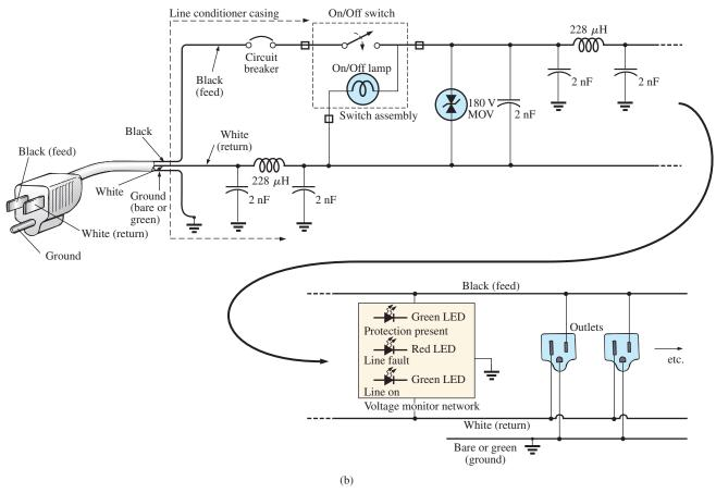
FIG. 10.79(b) Electrical schematic.
