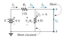
**FIG. 9.64** Determining  $I_N$  for the network in Fig. 9.62.
