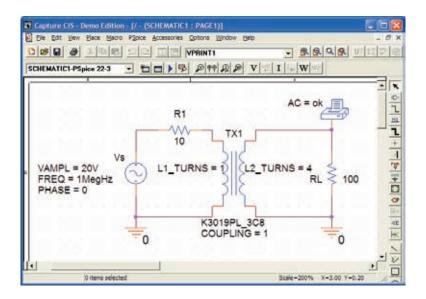
FIG. 22.53 Using a transformer provided in the EVAL library to analyze the network in Fig. 22.50.
