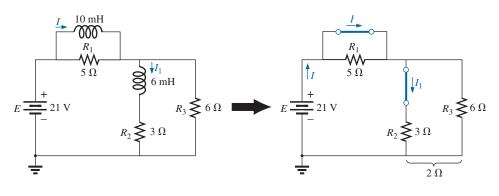
**FIG. 11.61** *Establishing the equivalent network for*  $t > 5\tau$ *.*
