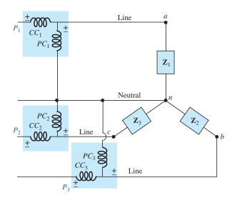
FIG. 23.28 Three-wattmeter method for a Y-connected load.
