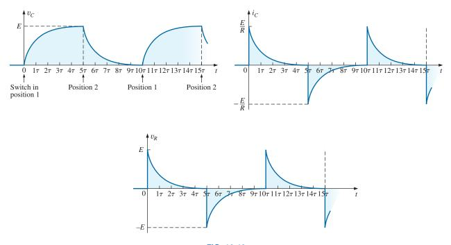
**FIG. 10.40**  $v_c$ ,  $i_c$ , and  $v_R$  for  $5\tau$  switching between contacts in Fig. 10.39(a).
