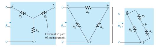
**FIG. 8.83** Finding the resistance  $R_{a,c}$  for the Y and  $\Delta$  configurations.
