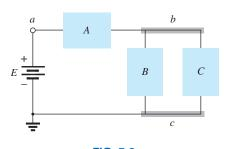
FIG. 7.8 Introducing the block diagram approach.
