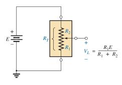
**FIG. 7.42** *Unloaded potentiometer.*
