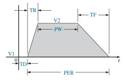
FIG. 10.82 The defining parameters of PSpice VPULSE.
