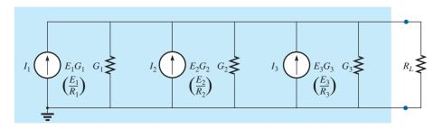
FIG. 9.92 Converting all the sources in Fig. 9.91 to current sources.
