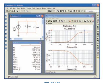
FIG. 15.119 Obtaining an impedance plot for a parallel R-L network using Multisim.
