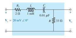
**FIG. 21.35** Series resonant pass-band filter for Example 21.8.
