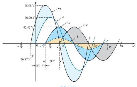
**FIG. 15.39** Waveforms for the series R-L-C circuit in Fig. 15.35.
