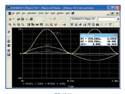
**FIG. 19.41** The resulting plots for the power, voltage, and current for the resistor in Fig. 19.40.
