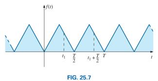
A waveform repetitive on the half-cycle.
