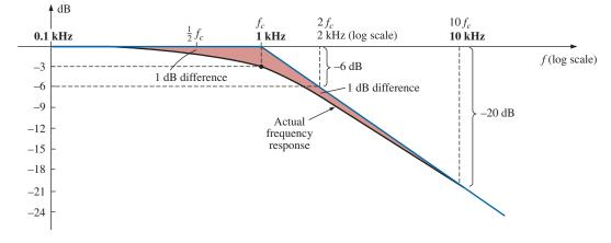
**FIG. 21.52** Bode plot for the high-frequency region of a low-pass R-C filter.
