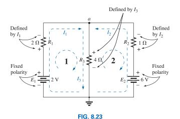
Inserting the polarities across the resistive elements as defined by the chosen branch currents.
