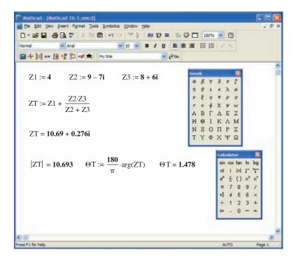
FIG. 16.20 Using Mathcad to determine the total impedance for the network in Fig. 16.18.
