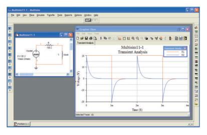
**FIG. 11.80** Using Multisim to obtain the transient response for an inductive circuit.
