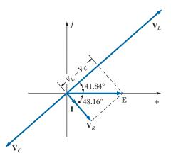
FIG. 15.45 Phasor diagram for the circuit in Fig. 15.43.
