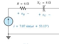
FIG. 15.30 Series R-C ac circuit.
