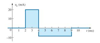
FIG. 11.55 Voltage across a 4 mH coil due to the current in Fig. 11.54.
