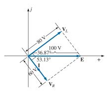
FIG. 15.29 Phasor diagram for the series R-L circuit in Fig. 15.26.
