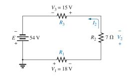
FIG. 5.32 Series configuration to be examined in Example 5.13.
