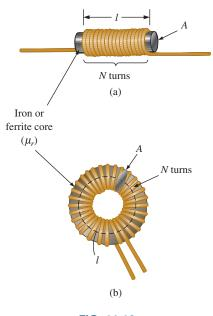
**FIG. 11.16** *Defining the parameters for Eq. (11.6).*
