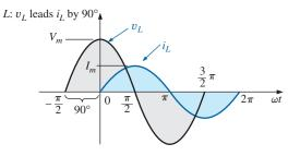
FIG. 14.9 For a pure inductor, the voltage across the coil leads the current through the coil by 90°.
