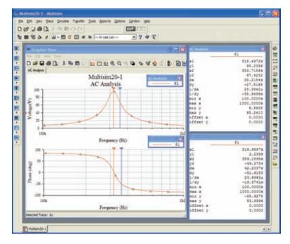
**FIG. 20.48** *Magnitude and phase plots for the voltage*  $v_C$  *of the network in Fig. 20.47.*
