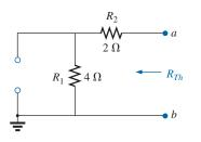
FIG. 9.34 Determining  $R_{Th}$  for the network in Fig. 9.33.
