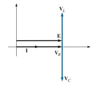
FIG. 20.3 Phasor diagram for the series resonant circuit at resonance.
