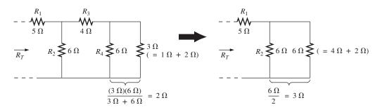
**FIG. 7.33** Working back to the source to determine  $R_T$  for the network in Fig. 7.32.
