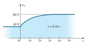
FIG. 10.63  $v_C$  for the network in Fig. 10.61.
