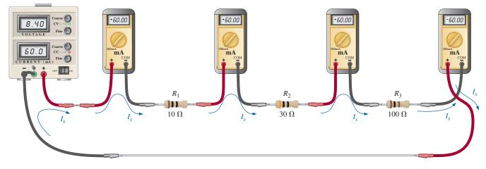
**FIG. 5.20** *Measuring the current throughout the series circuit in Fig. 5.12.*
