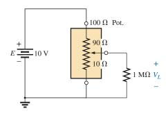
**FIG. 7.45** Loaded potentiometer with  $R_L \gg R_T$ .
