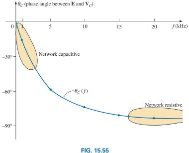
The phase angle between E and  $V_c$  versus frequency for the circuit in Fig. 15.47.
