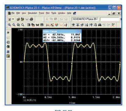
FIG. 25.27 The resulting waveform of the voltage across the resistor R in Fig. 25.26.
