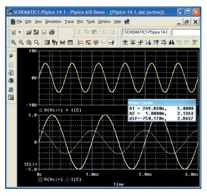
**FIG. 14.80** *A plot of the voltage, current, and power for the capacitor in Fig. 14.79.*
