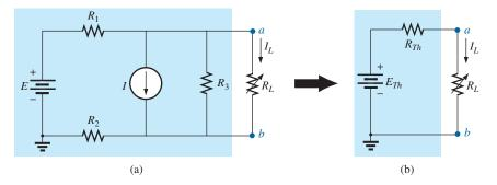
FIG. 9.25 Substituting the Thévenin equivalent circuit for a complex network.
