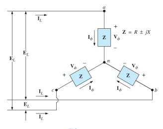
FIG. 23.22 Y-connected balanced load.
