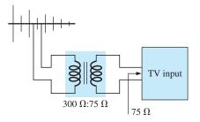
**FIG. 22.9** *Television impedance matching transformer.*
