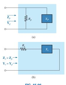
FIG. 15.96 Defining the parameters of equivalent series and parallel networks.
