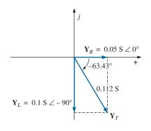
**FIG. 15.62** Admittance diagram for the network in Fig. 15.60.
