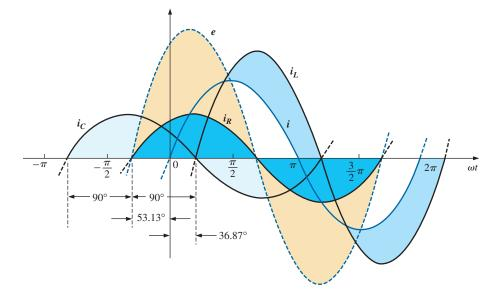
FIG. 15.81 Waveforms for the parallel R-L-C network in Fig. 15.77.
