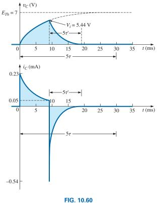
The resulting waveforms for the network in Fig. 10.57.
