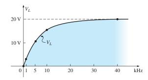
**FIG. 15.57** Plotting  $V_L$  versus f for the series R-L circuit in Fig. 15.56.
