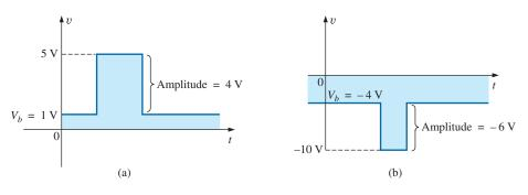
**FIG. 24.3** *Defining the base-line voltage.*
