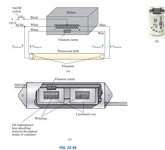
(a) Schematic of single-bulb fluorescent lamp; (b) starter; (c) internal view of ballast transformer.
