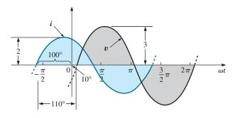
**FIG. 13.33** *Example 13.12(c): i leads v by 110°.*
