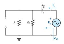
FIG. 18.50 Determining the Thévenin impedance using the approach  $\mathbf{Z}_{Th} = \mathbf{E}_g / \mathbf{I}_g$ .
