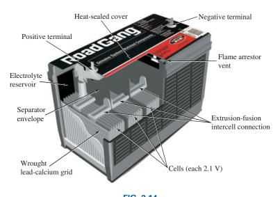
FIG. 2.14 Maintenance-free 12 V (actually 12.6 V) lead-acid battery. (Courtesy of Remy International, Inc.)
