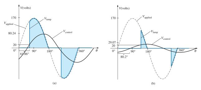
**FIG. 15.115** Light dimmer in Fig. 11.68; (a) rheostat set at 33 k $\Omega$ ; (b) rheostat set at 200 k $\Omega$ .
