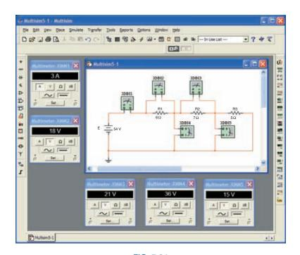
FIG. 5.84 Applying Multisim to a series dc circuit.
