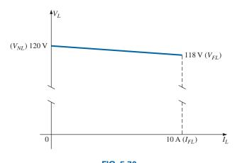
FIG. 5.70 Terminal characteristics for the supply of Example 5.28.
