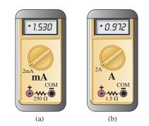
FIG. 5.73 Including the effects of the internal resistance of an ammeter: (a) 2 mA scale; (b) 2 A scale.
