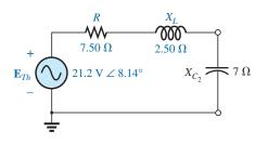
FIG. 18.74 The Thévenin equivalent circuit for the network in Fig. 18.67.
