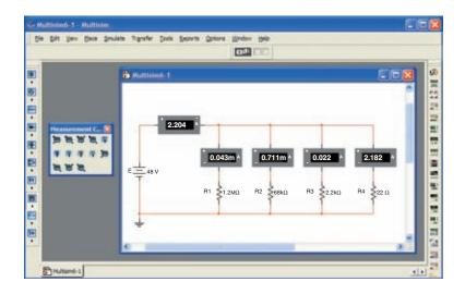
FIG. 6.71 Using the indicators of Multisim to display the currents of a parallel dc network.
