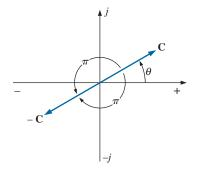
FIG. 14.44 Demonstrating the effect of a negative sign on the polar form.
