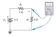
**FIG. 9.30** *Measuring*  $E_{Th}$  *for the network in Fig. 9.27.*
