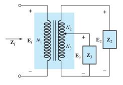
FIG. 22.44 Ideal transformer with a tapped secondary and multiple loads.
