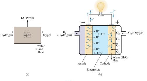
**FIG. 2.21** Fuel cell (a) components; (b) basic construction.
