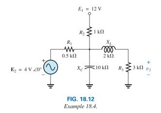
**Solution:** For the dc analysis, the capacitor can be replaced by an opencircuit equivalent, and the inductor by a short-circuit equivalent. The result is the network in Fig. 18.13.
