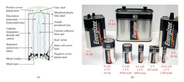
FIG. 2.12 Alkaline primary cell: (a) Cutaway of cylindrical Energizer® cell; (b) various types of Eveready Energizer® primary cells. (© Eveready Battery Company, Inc., St. Louis Missouri)
