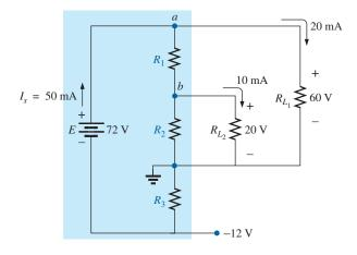
**FIG. 7.41** *Voltage divider supply for Example 7.12.*
