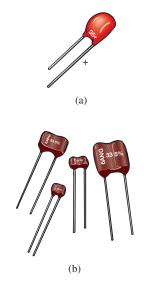
FIG. 10.18 Dipped capacitors: (a) polarized tantalum; (b) nonpolarized mica.
