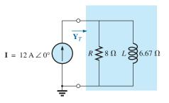
**FIG. 15.103** *Parallel equivalent of the circuit in Fig. 15.102.*
