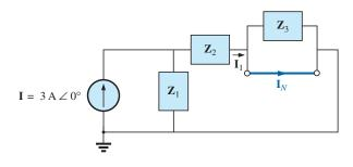
**FIG. 18.71** Determining  $I_N$  for the network in Fig. 18.67.
