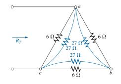
FIG. 8.94 Substituting the converted Y configuration into the network in Fig. 8.91.
