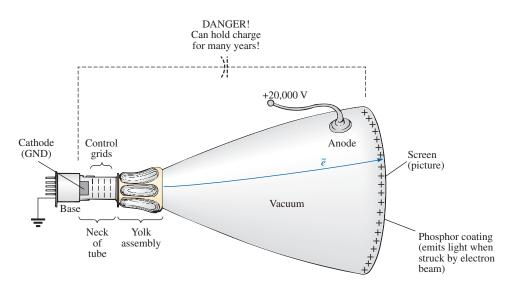
**FIG. 11.70** *Yolk assembly for a TV or PC tube.*
