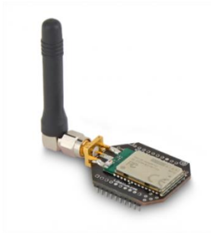
Fig. 3.7 Bluetooth Modules for Arduino plugged into the XBee Shield.
