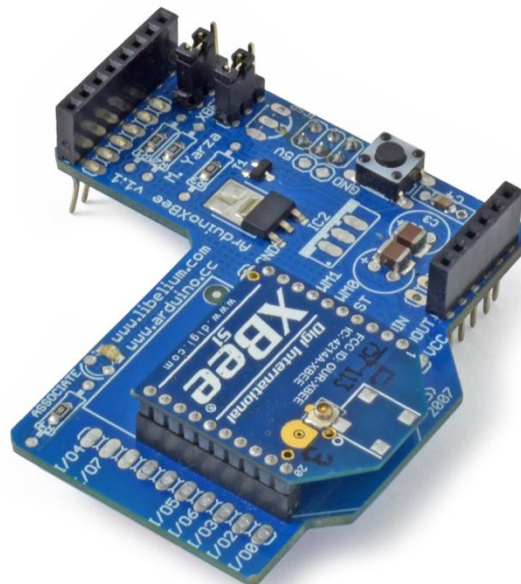
Fig. 3.6 Xbee Module attached to Xbee Shield
